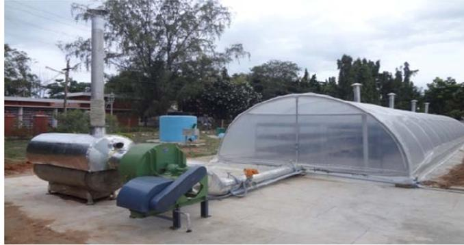
Renewable energy integrated drying system using solar thermal and biomass hot air with controlled environment can be used for continuous drying of agro-products.
