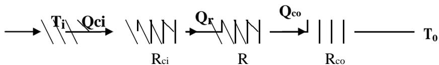
**Thermal circuit for a hollow sphere with convective boundary conditions 3.12**
