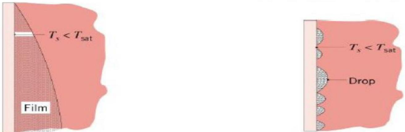
Fig. 1 Film-wise and drop-wise condensation
