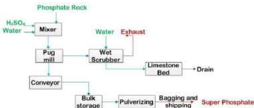
Figure: Manufacturing of Superphosphate
