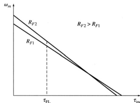
Some small DC motors used in control circuits may operate at speeds close to stall conditions. For such motors, an increase in field resistance may have no effect (or opposite to the expected effect) on the motor speed. The result of speed control by field resistance is not predictable and, thus, this type of control is not very common.
