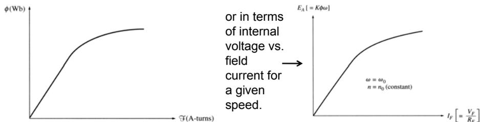
To get the maximum possible power per weight out of the machine, most motors and generators are operating near the saturation point on the magnetization curve. Therefore, when operating at full load, often a large increase in current  $I_F$  may be needed for small increases in the generated voltage  $E_A$ .
