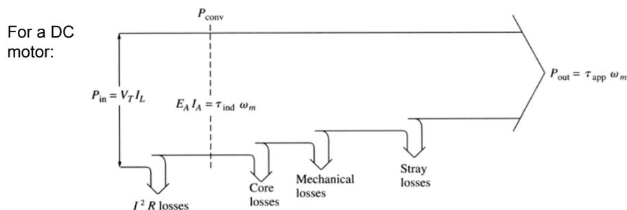
Electrical power is input to the machine, and the electrical and brush losses must be subtracted. The remaining power is ideally converted from electrical to mechanical form at the point labeled as  $P_{conv}$ .
