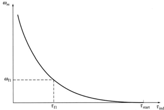
Steps must be taken to ensure that a series motor **always** has a load! Therefore, it is not a good idea to connect such motors to loads by a belt or other mechanism that could break.
