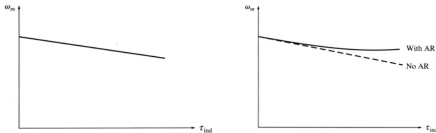
However, if a motor has an armature reaction, flux-weakening reduces the flux when torque increases. Therefore, the motor's speed will increase. If a shunt (or separately excited) motor has compensating windings, and the motor's speed and armature current are known for any value of load, it's possible to calculate the speed for any other value of load.
