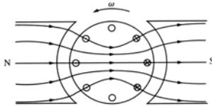
The effect of the air gap on the pole flux.
