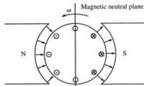
A two-pole DC machine: initially, the pole flux is uniformly distributed and the magnetic neutral plane is vertical.
