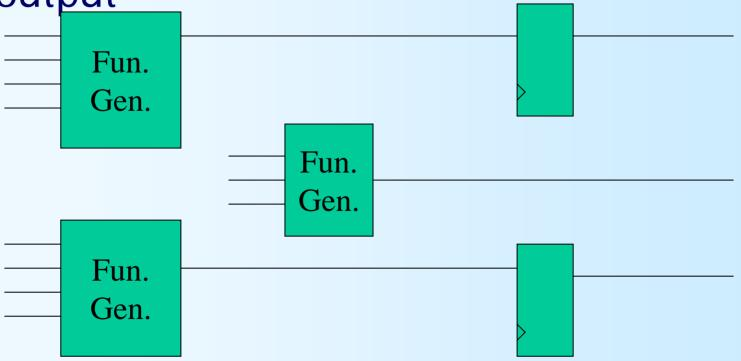
One 9-input function generatorLatched or unlatched output
