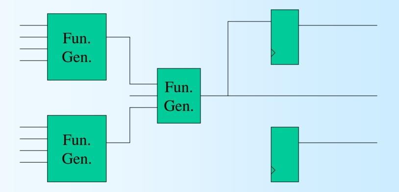
One 9-input function generatorLatched or unlatched output
