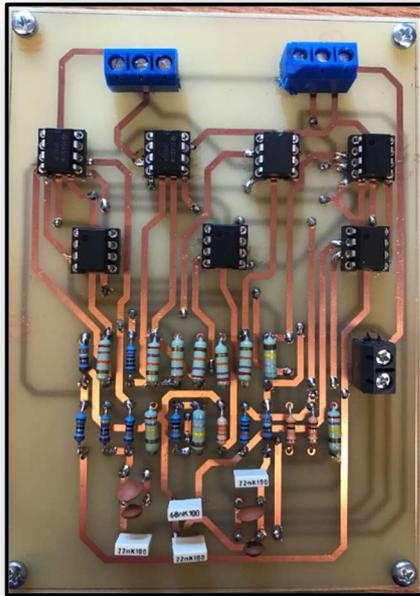
**Figure 10. Upper layer of the PCB**
