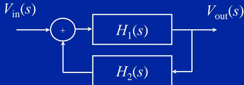
Linear model of an oscillator as a feedback control system.
