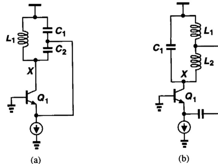
Figure 7.7 (a) Colpitts and (b) Hartley oscillators.
