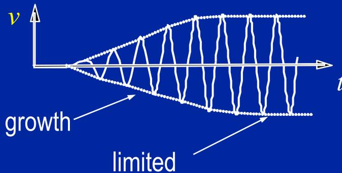
Waveform of an LC resonator with losses compensated. The oscillation grows until a practical constraint limits the amplitude.
