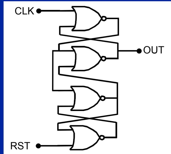
Positive edge-triggered D flip-flop with active low reset and hidden  $D=1$
