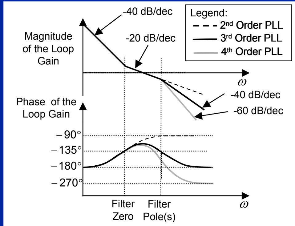
Comparison of open loop gain and phase in a second, third, and fourth order PLL
