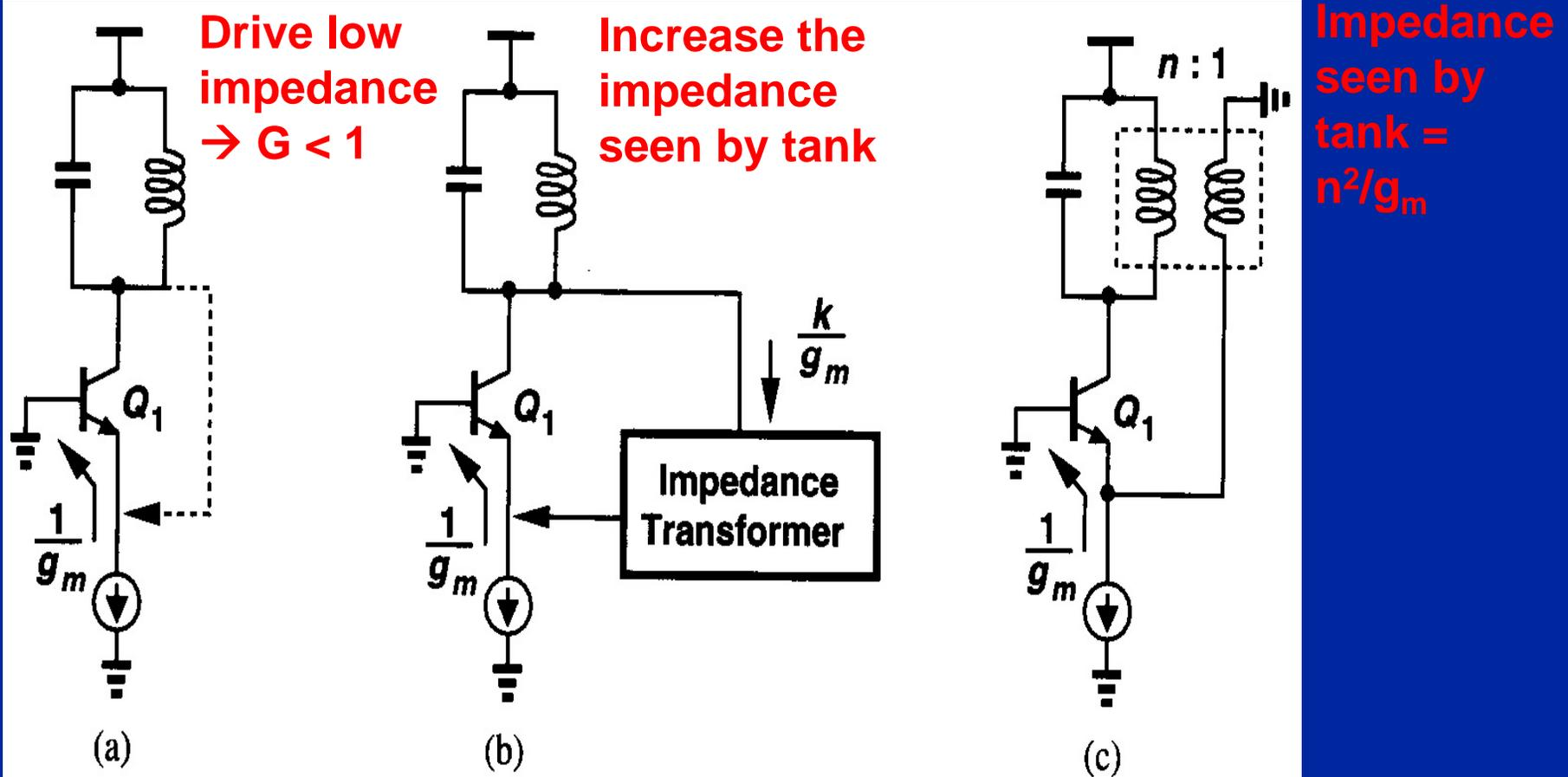
**Figure 7.6** (a) Direct feedback from collector to emitter, (b) insertion of an impedance transformer, (c) use of an explicit transformer.
