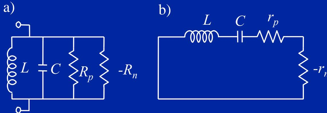
The addition of negative resistance to the circuit to overcome losses in a) a parallel resonator or b) a series resonator.
