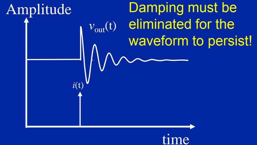
Damped LC resonator with current step applied.
