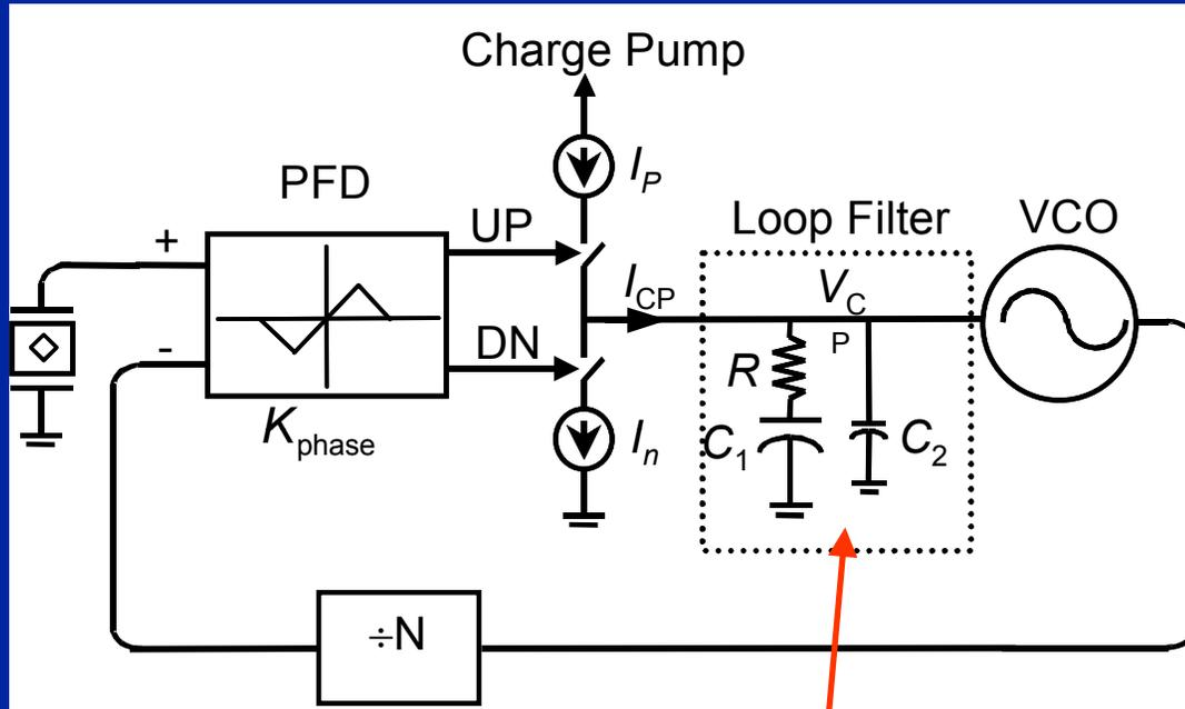
The 2nd-order filter is the highest order passive RC filter that can be built without series resistors between the charge pump and the VCO tune line
