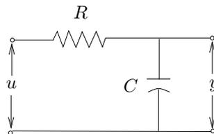
Figure 4.1: A low-pass filter.
