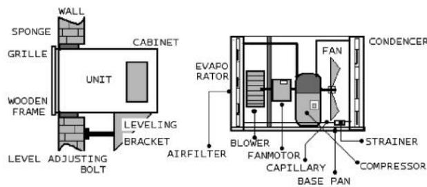
This type of AC is designed to fit into the window sills. A single unit of Window Air Conditioner houses all the necessary components, namely the compressor, condenser, expansion valve or coil, evaporator and cooling coil enclosed in a single box. Since the window AC is a single unit, it takes less effort to install as well as maintain.
