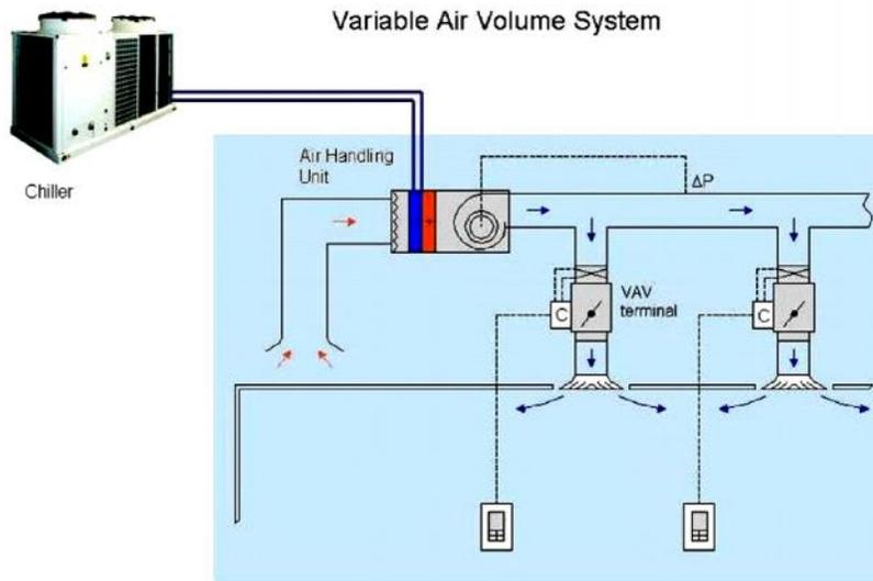
**Variable Air Volume (VAV)** is a type of heating, ventilating, and/or air-conditioning (HVAC) system. Unlike constant air volume (CAV) systems, which supply a constant airflow at a variable temperature, VAV systems vary the airflow at a constant temperature. The advantages of VAV systems over constant-volume systems include more precise temperature control, reduced compressor wear, lower energy consumption by system fans, less fan noise, and additional passive dehumidification.
