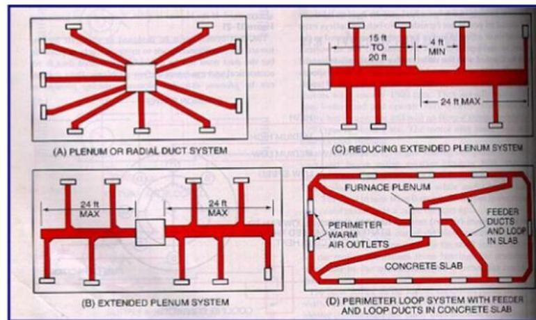
(A) Plenum system. (B) Extended plenum system.
