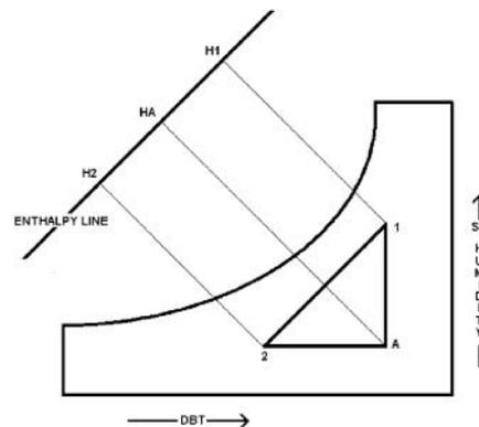
Sensible heat gain due to in filtered air =  $m ( H_A - H_2 )$
