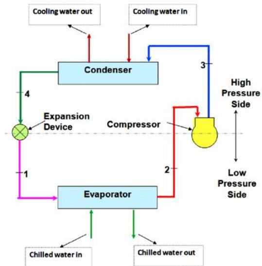
A *chiller* is a machine that removes heat from a liquid via vapour-compression or absorption refrigeration cycle. This liquid can then be circulated through a heat exchanger to cool air or equipment as required.
