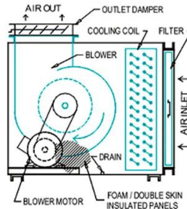
a roof or in large mechanical rooms located in the building. They often have an economizer or inlet damper that allows small amount of outside air or make-up air to be pulled in through the air handler. There are several types of Air Handling Units: Compact, Modular, Residential, DX integrated, Low Profile (ceiling), Packaged, Rooftop mounted (typically on the roofs of buildings, with special weather protection), etc.
