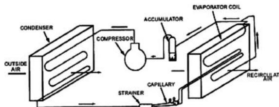
This unit has a double shaft fan motor with fans mounted on either side of the motor. One at the evaporator side and the other at the condenser side. The evaporator side is located facing the room for cooling the space and the condenser side outdoor for heat rejection. There is an insulated partition separating the two sides within the same casing.
