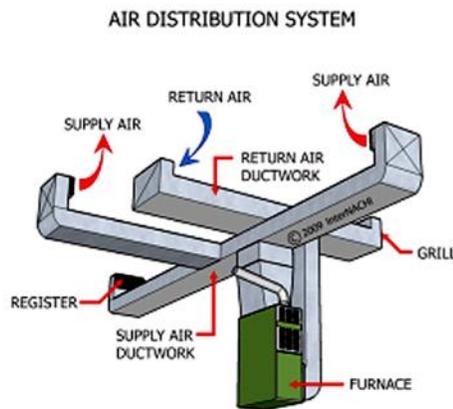
In air conditioning systems the ‘duct’ is considered a static component of the installation through which air flows within the building, connecting all parts of the system and via used or exhaust air is discharged.
