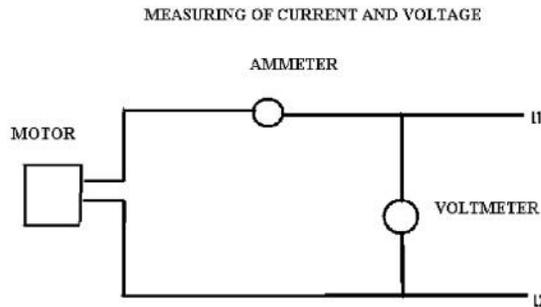
**AMMETER** : It is used to measure current in a circuit.
