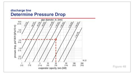
After the pipe diameter is selected, the overall pressure drop due to the discharge line can be calculated. The next step is to calculate the total "equivalent" length of the straight pipe and fittings. The equivalent length data for copper fittings used in the discharge line is the same as for the suction line.
