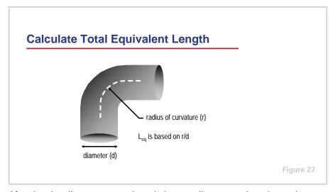
After the pipe diameters are selected, the overall pressure drop due to the suction line can be calculated. The next step is to calculate the total "equivalent" length of the suction line. The total equivalent length is the actual measured length of straight pipe plus the pressure drop through any fittings, such as elbows and tees. The pressure drop through the fittings is expressed in terms of the length of straight pipe that would produce the same pressure drop.
