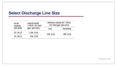
Based on the minimum allowable velocities listed in Figure 45 on page 35, 1 5/8 in. (42 mm) is the largest diameter of pipe that will result in acceptable velocity, at both maximum and minimum capacities, within horizontal and vertical drop sections.
