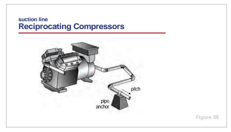
Finally, when the system includes a reciprocating compressor, an anchored, 45-degree canted loop should be constructed very close to the location at which the suction line connects to the compressor. This loop absorbs vibration generated by the reciprocating motion of the compressor, minimizing the amount of vibration transmitted to the piping system.
