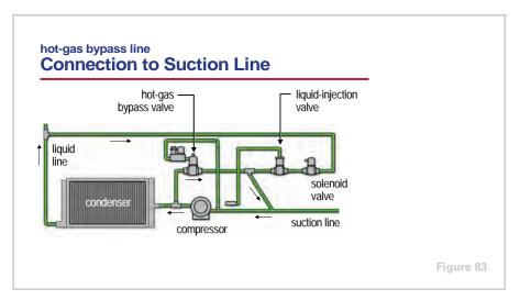
Again, routing of the hot-gas bypass piping is critical. Install the hot-gas bypass valve above the compressor discharge and close to the compressor. Pitch the section of pipe between the discharge line and the hot-gas bypass valve so that oil will drain back into the discharge line. Tap the pilot line for the hot-gas bypass valve close to the compressor inlet, and pitch the piping downstream of the hot-gas bypass valve so that oil will drain away from the valve, toward the suction line.
