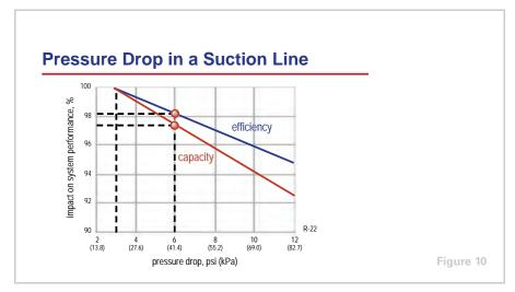
The third requirement of the refrigerant piping design is to minimize system capacity loss. To achieve the maximum capacity from the system, the refrigerant must circulate through the system as efficiently as possible. This involves minimizing any pressure drop through the piping and other system components.
