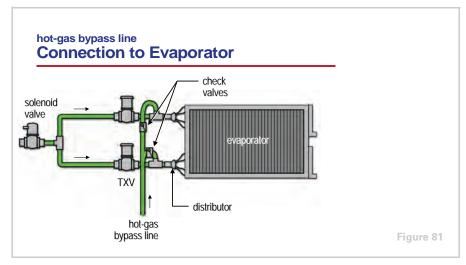
The evaporator shown in Figure 81 also contains two distributors on a single refrigeration circuit, but it only contains one solenoid valve. In this example, the solenoid valve closes only after the last compressor on the circuit shuts off. Both distributors are "active" at all times and the hot-gas bypass pipe must be connected to both distributors.
