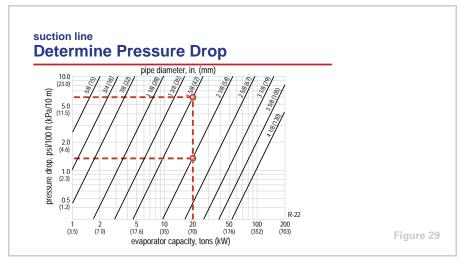
The next step is to determine the pressure drop due to the straight pipe and fittings, based on the calculated total equivalent length. The chart in Figure 29 shows the pressure drop, per unit of equivalent length, for different pipe diameters and various system capacities. At the maximum capacity of 20 tons (70.3 kW), the pressure drop due to the 2 1/8 in. (54 mm)-diameter sections of straight pipe and fittings is 1.4 psi per 100 ft of equivalent length (3.2 kPa/10 m), or 0.93 psi (6.4 kPa).
