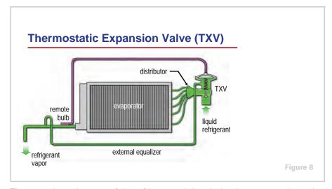
The second requirement of the refrigerant piping design is to ensure that only liquid refrigerant enters the expansion device. There are several types of expansion devices, including expansion valves (thermostatic or electronic), capillary tubes, and orifices.
