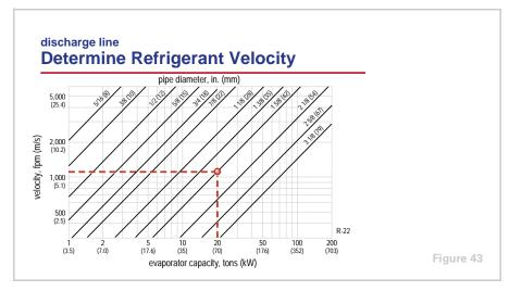
The chart in Figure 43 shows the velocity of R-22 inside discharge pipes of various diameters at one particular operating condition—40°F (4.4°C) saturated suction temperature, 125°F (51.7°C) saturated condensing temperature, 12°F (6.7°C) of superheat, 15°F (8.3°C) of subcooling, and 70°F (38.9°C) of compressor superheat.
