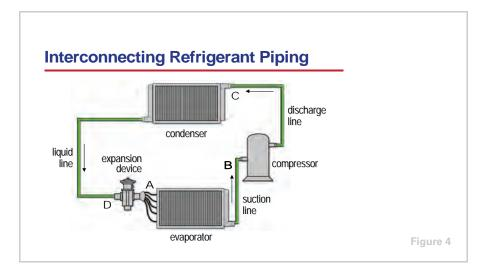
These individual components are connected by refrigerant piping. The suction line connects the evaporator to the compressor, the discharge line connects the compressor to the condenser, and the liquid line connects the condenser to the expansion device. The expansion device is typically located at the end of the liquid line, at the inlet to the evaporator.
