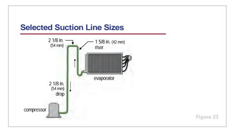
For this example system, a 2 1/8 in. (54 mm)-diameter pipe can be used for the horizontal and vertical drop sections of the suction line, and a 1 5/8 in. (42 mm)-diameter pipe should be used for the vertical riser. This combination of pipe sizes will ensure proper oil movement at both maximum and minimum system capacities, and minimize the overall pressure drop due to the suction line.
