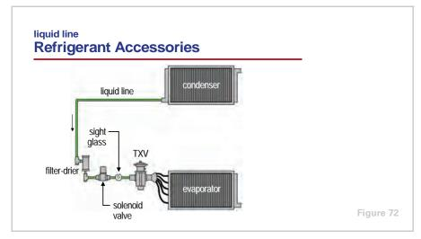
For proper refrigerant distribution into the evaporator coil, one TXV is required for each distributor.
