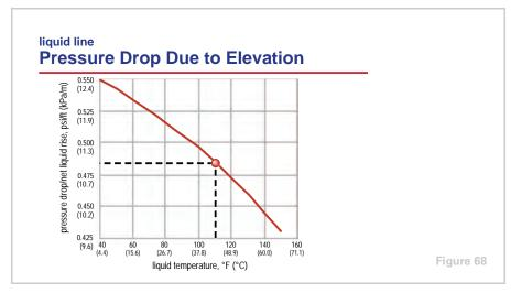
The chart in Figure 68 shows that the magnitude of the associated pressure drop (or gain) depends primarily on the temperature (density) of the liquid refrigerant. The greatest pressure drop (or gain) due to this vertical column of liquid occurs when the temperature of the liquid refrigerant is the lowest.
