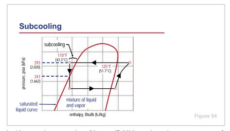
In this example system, the refrigerant (R-22) is condensed at a temperature of 125°F (51.7°C), which corresponds to a pressure of 293 psia (2,020 kPa). Inside the subcooling tubes, the temperature of the liquid refrigerant is reduced by 15°F (8.3°C) to 110°F (43.3°C). Ignoring the pressure drop due to the condenser and subcooler tubes, the pressure of this subcooled liquid refrigerant is the same, 293 psia (2,020 kPa).
