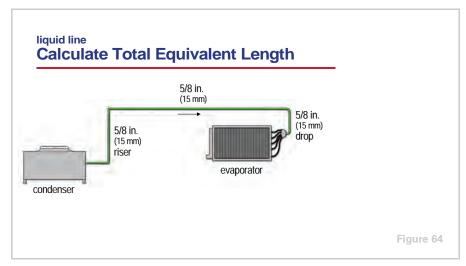
The next step is to calculate the total equivalent length by adding the actual measured length of straight pipe to the equivalent length of any fittings to be installed in the liquid line. The equivalent length data for copper fittings used in the liquid line is the same as for the suction and discharge lines.
