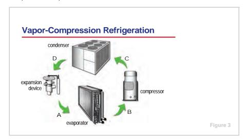
Figure 3 illustrates a basic vapor-compression refrigeration cycle. Refrigerant enters the evaporator in the form of a cool, low-pressure mixture of liquid and vapor (A). Heat is transferred to the refrigerant from the relatively warm air that is being cooled, causing the liquid refrigerant to boil. The resulting refrigerant vapor (B) is then pumped from the evaporator by the compressor, which increases the pressure and temperature of the vapor.
