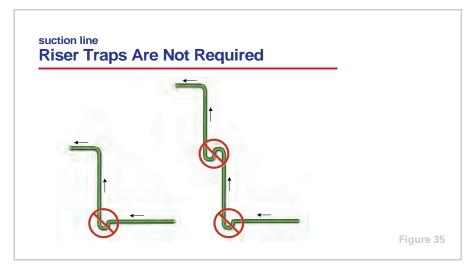
As mentioned earlier, the trap shown in Figure 32 on page 25, and Figure 33 on page 26, is used to provide free drainage from the evaporator and section of pipe to which the TXV bulb is attached. Its purpose is *not* to drain the suction riser
