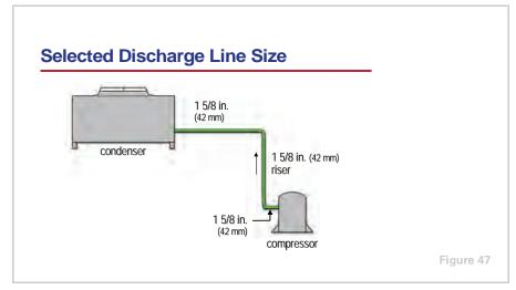
For this example system, a 1 5/8 in. (42 mm)-diameter pipe can be used for all horizontal and vertical sections of the discharge line, including vertical risers. This pipe size will ensure proper oil movement at both maximum and minimum system capacities, and minimize the overall pressure drop due to the discharge line.
