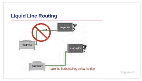
How the liquid line is routed can be important, particularly when the condenser is located below the evaporator. As an example, the upper system in Figure 73 routes the liquid-line riser *before* a long horizontal run. The lower system routes the riser *after* a long horizontal run.
