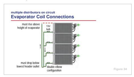
When an evaporator has more than one distributor connected to a single refrigeration circuit, there are some additional considerations for manifolding the suction headers into a single suction line.
