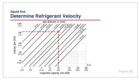
The chart in Figure 62 shows the velocity of liquid R-22 inside liquid lines of various diameters at one particular operating condition—40°F (4.4°C) saturated suction temperature, 125°F (51.7°C) saturated condensing temperature, 12°F (6.7°C) of superheat, 15°F (8.3°C) of subcooling, and 70°F (38.9°C) of compressor superheat.
