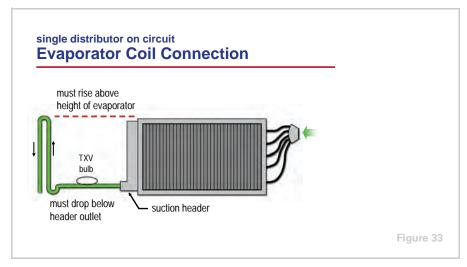
If the suction line leaves the evaporator and then must drop vertically, an inverted trap is used to prevent refrigerant and oil inside the evaporator from free draining into the suction line, and toward the compressor, when the system is off.
