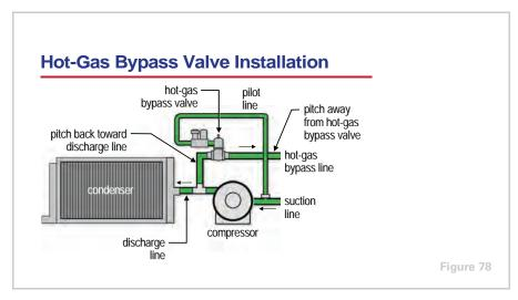
Due to the widely varying velocity in the hot-gas bypass line, the selected diameter of the pipe is not as critical as its routing. Install the **hot-gas bypass**
