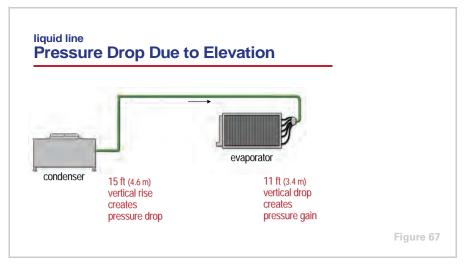
The next step is to calculate the loss of subcooling due to the liquid-line pressure drop and any elevation change.
