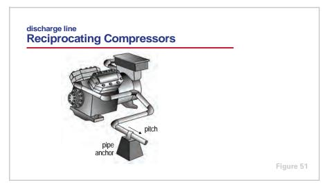
Finally, when the system includes a reciprocating compressor, an anchored, 45-degree canted loop should be constructed very close to the location at which the discharge line connects to the compressor. This loop absorbs vibration generated by the reciprocating motion of the compressor. Note that the loop is pitched downward to provide free drainage away from the compressor.
