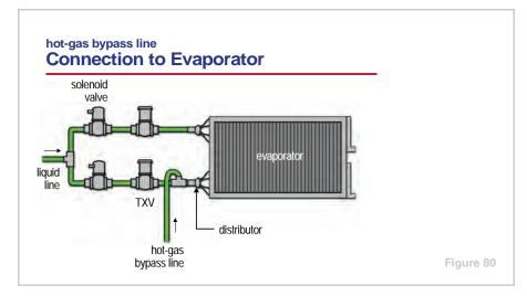
The hot-gas bypass line is then piped to the evaporator inlet. It must be connected to the top of the pipe, between the TXV and the distributor. Any hot-gas bypass piping upstream of this connection should be pitched so that oil or condensed refrigerant will drain toward the evaporator.
