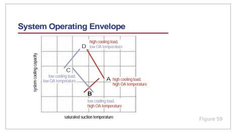
This operating envelope defines four extreme corners. Condition **A** depicts the system operating with a high cooling load at a high outdoor temperature, and condition **B** depicts a low cooling load at the same high outdoor temperature. Condition **C** depicts the system operating with a low cooling load at a low outdoor temperature, and condition **D** depicts a high cooling load at the same low outdoor temperature.
