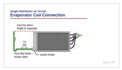
After this short horizontal section, the suction line should drop vertically downward to allow the evaporator, and the section of pipe with the TXV bulb attached, to drain freely when the system is operating.
