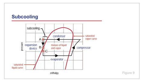
Inside the condenser, after all of the refrigerant vapor has condensed into liquid, the refrigerant is subcooled to further lower its temperature. This subcooled liquid refrigerant leaves the condenser (**A**) and experiences a pressure drop as it flows through the liquid line and accessories, such as a filter
