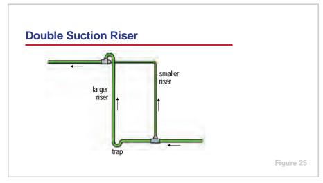
A double suction riser is constructed of a larger-diameter riser with a trap at the base and a smaller-diameter riser in parallel. At maximum capacity, the refrigerant vapor flows up both risers at velocities that are adequate to carry the oil droplets.
