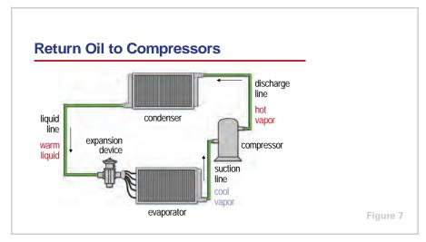
Returning to the system schematic, droplets of oil are pumped out of the compressor along with the hot, high-pressure refrigerant vapor. The velocity of the refrigerant inside the discharge line must be high enough to carry the small oil droplets through the pipe to the condenser.
