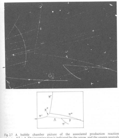
Fig. 2.7 A bubble chamber picture of the associated production reaction  $\pi^- + p \rightarrow K^0 + \Lambda$ . The incoming pion is indicated by the arrow, and the unseen neutrals are detected by their decays  $K^0 \rightarrow \pi^+ + \pi^-$  and  $\Lambda \rightarrow \pi^- + p$ . This picture was taken in the 10 inch (25 cm) bubble chamber at the Lawrence Berkeley Radiation Laboratory. (Photograph courtesy of the Lawrence Berkeley Radiation Laboratory.)
