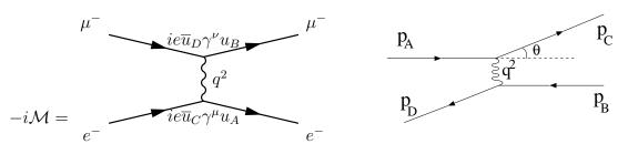
Figure 8.2:  $e^-\mu^- \to e^-\mu^-$  scattering. left: the Feynman diagram. right: the scattering process.
