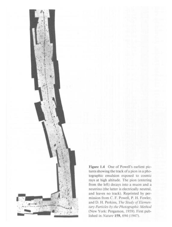
Figure 1.3: A pion entering from the left decays into a muon and an invisible neutrino.
