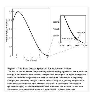
Figure 1.2: The beta spectrum as observed in tritium decay to helium. The endpoint of the spectrum can be used to set a limit of the neutrino mass. *Question: how?*
