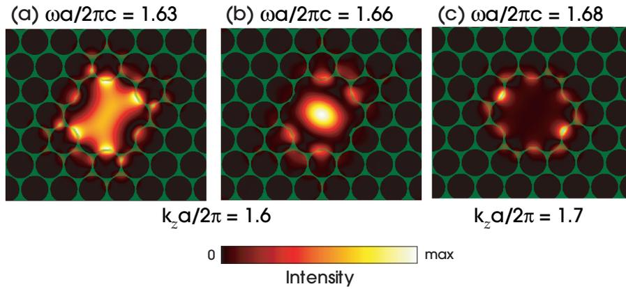
**Figure 11:** Intensity patterns ( $\hat{z} \cdot \text{Re}[\mathbf{E}^* \times \mathbf{H}]$ ) of three doubly degenerate modes of a hollow-core holey fiber ( $\epsilon$  shaded green), corresponding to the dots on the thick red lines in figure 10. (a) and (b) lie above the air light line at  $k_z a/2\pi = 1.6$ , while (c) is a surface state lying below the air light line at  $k_z a/2\pi = 1.7$ .
