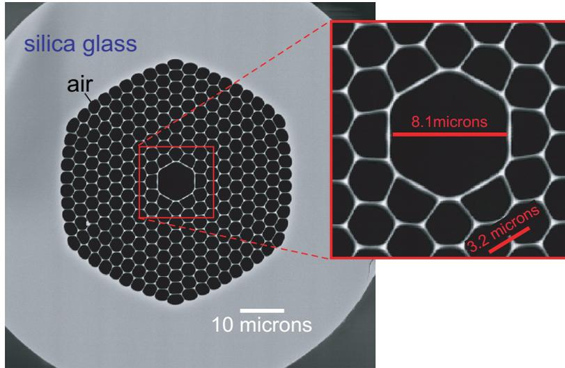
**Figure 9:** Electron-microscope image of hollow-core holey-fiber cross section (black regions are air holes, and gray regions are silica glass). Central air defect, replacing 7 holes, supports gap-guided modes around a wavelength of 1060 nm. (Image courtesy Karl Koch and Corning, Inc.)
