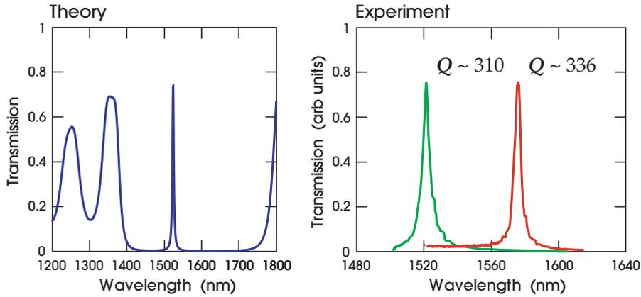
**Figure 9:** Theoretical and experimental transmission spectra (versus vacuum wavelength) for air-bridge filter of figure 8. *Left:* Theory, showing transmission peak in gap and broad Fabry–Perot oscillations outside gap. *Right:* Experiment, showing transmission for two defect separations  $d = 1.26a$  (left,  $Q = 310$ ) and  $d = 1.41a$  (right,  $Q = 336$ ).
