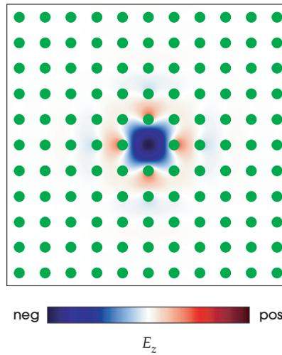
**Figure 3:** Point-defect cavity formed by a single missing rod in a square lattice of radius  $0.2a$  dielectric rods ( $\epsilon = 11.4$ ) in air. The cavity supports a single mode of frequency  $\omega a / 2\pi c = 0.38$ , inside the TM band gap, whose electric field  $E_z$  is shown.
