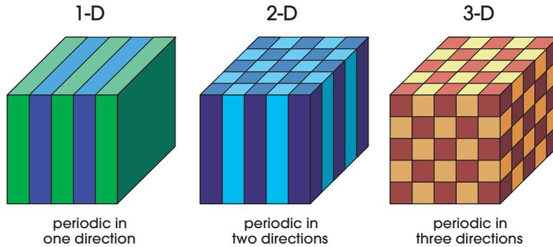
**Figure 1:** Simple examples of one-, two-, and three-dimensional photonic crystals. The different colors represent materials with different dielectric constants. The defining feature of a photonic crystal is the periodicity of dielectric material along one or more axes.
