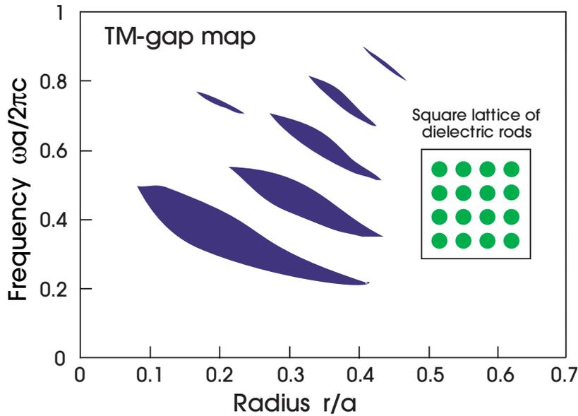
**Figure 1:** “Gap map” showing TM gap locations versus rod radius for a square lattice of dielectric rods ( $\epsilon = 11.4$ ) in air (inset).
