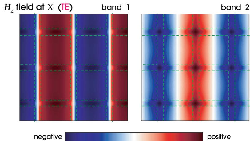
**Figure 7:** Magnetic fields of X-point TE modes for a square array of dielectric ( $\epsilon = 8.9$ ) veins in air. The green dashed lines indicate the veins, and the color indicates the amplitude of the magnetic field (which is oriented in the  $z$  direction). The dielectric band is on the left, and the air band is on the right.
