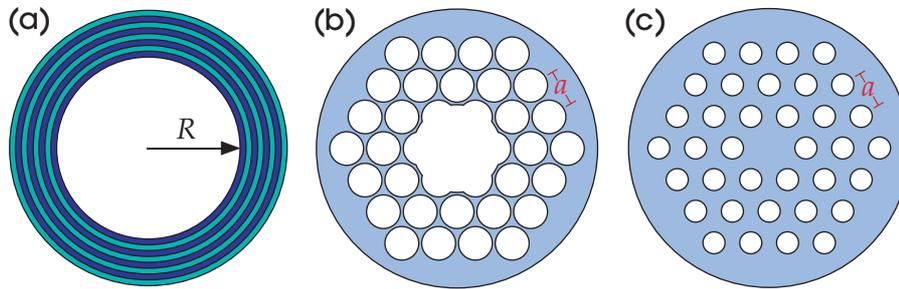
**Figure 1:** Three examples of photonic-crystal fibers. (a) Bragg fiber, with a one-dimensionally periodic cladding of concentric layers. (b) Two-dimensionally periodic structure (a triangular lattice of air holes, or “holey fiber”), confining light in a hollow core by a band gap. (c) Holey fiber that confines light in a solid core by index guiding.
