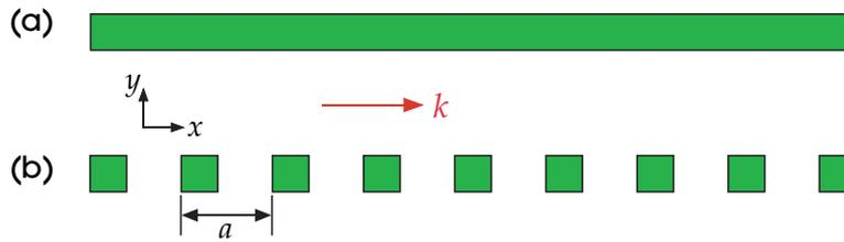
**Figure 2:** (a) Two-dimensional dielectric waveguide ( $\epsilon = 12$ ) of width  $0.4a$ . (b) Periodic waveguide: a period- $a$  sequence of  $0.4a \times 0.4a$  dielectric squares. In both (a) and (b) there is a conserved wave vector  $k$  along the direction  $x$  of translational symmetry, resulting in guided modes.
