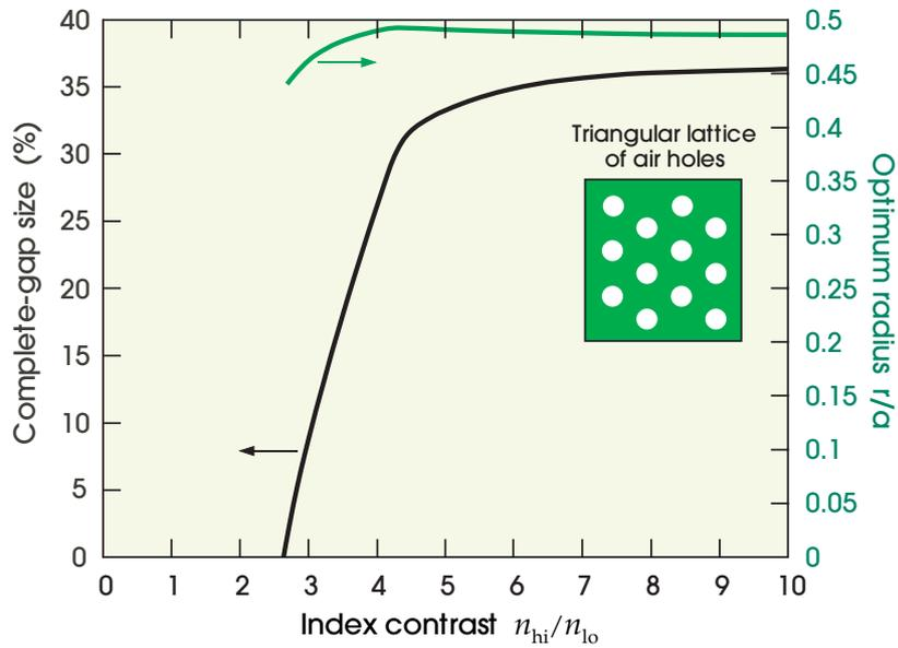
**Figure 8:** Gap recipe for the lowest *complete* gap of the triangular lattice of air holes in dielectric.
