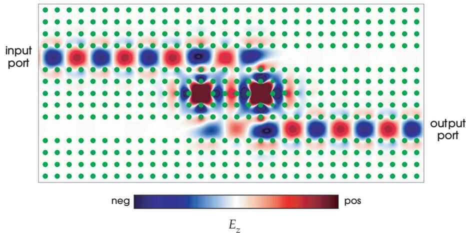
**Figure 13:** A **channel-drop filter** redirects 100% of light from the input port to the output port, but only around a single resonant frequency. Other frequencies propagate along the top waveguide unimpeded.  $E_z$  field at resonance is shown. This relies on a degenerate *pair* of resonant modes (here created by two missing-rod cavities), with appropriate symmetries, that couple the two waveguides.
