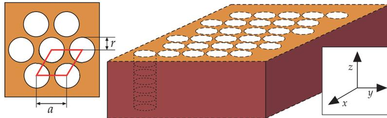
**Figure 8:** A two-dimensional photonic crystal of air columns in a dielectric substrate (which we imagine to extend indefinitely in the  $z$  direction). The columns have radius  $r$  and dielectric constant  $\epsilon=1$ . The left inset shows a view of the triangular lattice from above, with the unit cell framed in red. It has lattice constant  $a$ .
