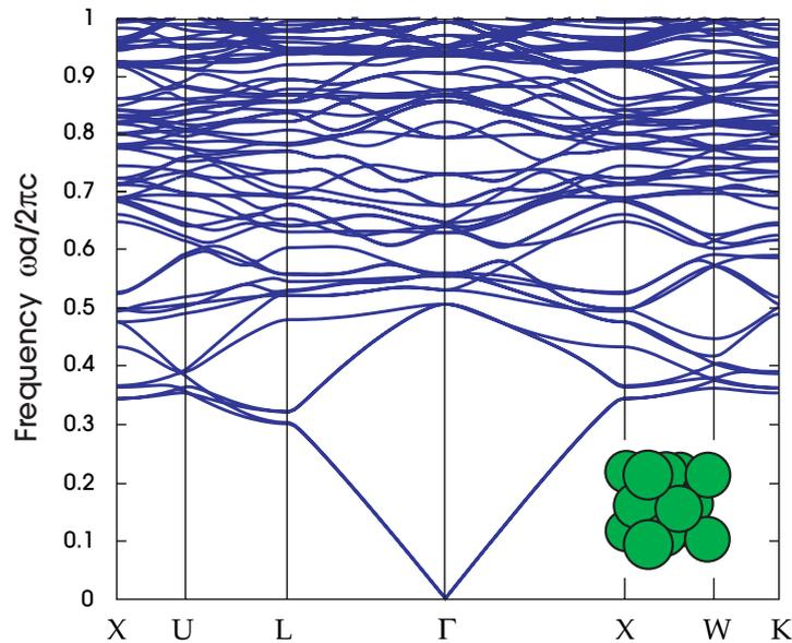
**Figure 2:** The photonic band structure for the lowest-frequency electromagnetic modes of a face-centered cubic (fcc) lattice of close-packed dielectric spheres ( $\epsilon = 13$ ) in air (inset). Note the *absence* of a complete photonic band gap. The wave vector varies across the irreducible Brillouin zone between the labelled high-symmetry points; see appendix B for a discussion of the Brillouin zone of an fcc lattice.
