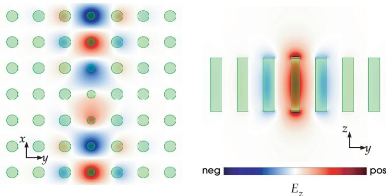
**Figure 6:**  $E_z$  field cross sections in reduced-radius line-defect waveguide from figure 5, for a defect rod radius of  $r = 0.14a$  at a wave vector  $k_x a / 2\pi = 0.42$ . The dielectric material is shaded translucent green. *Left:* horizontal ( $z = 0$ ) cross section (in which  $E_z$  is the only nonzero electric-field component). *Right:* vertical ( $x = 0$ ) cross section bisecting the rods perpendicular to the waveguide. The field decays exponentially away from the waveguide.
