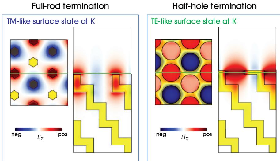
**Figure 20:** Horizontal and vertical cross sections (intersecting at green lines) of field patterns for the two crystal terminations from figure 19, at the K point. Dielectric material is shown in yellow. *Left:*  $E_z$  for “TM-like” band when the surface is terminated with a full rod layer. *Right:*  $H_z$  for “TE-like” band when the surface is terminated with half of a hole layer.
