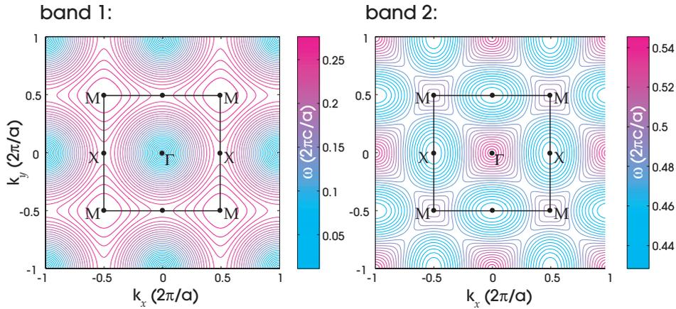
**Figure 15:** Isofrequency diagrams: contour plots of  $\omega(k_x, k_y)$  for the first two TM bands of a square lattice of radius  $0.2a$  dielectric rods ( $\epsilon = 11.4$ ) in air. The first Brillouin zone is shown as black squares.
