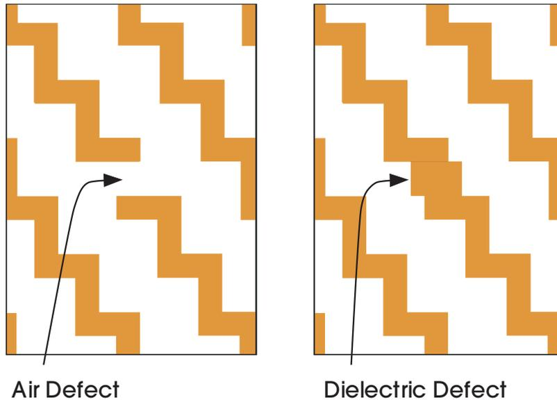
**Figure 13:** Vertical cross section of the layered structure from figure 10, corresponding to the top panel of figure 12, showing examples of how a point defect may be created by modifying a *single rod*: a rod can be removed (left) to form an **air defect**, or the radius of a rod can be increased (right) to form a **dielectric defect**.
