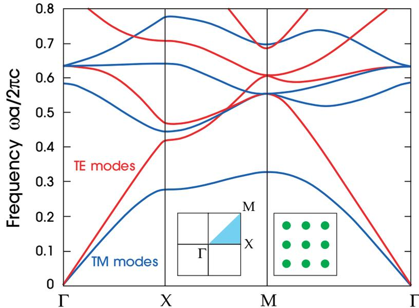
**Figure 2:** The photonic band structure for a square array of dielectric columns with  $r = 0.2a$ . The blue bands represent TM modes and the red bands represent TE modes. The left inset shows the Brillouin zone, with the irreducible zone shaded light blue. The right inset shows a cross-sectional view of the dielectric function. The columns ( $\epsilon = 8.9$ , as for alumina) are embedded in air ( $\epsilon = 1$ ).
