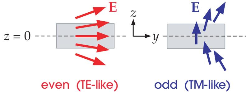
**Figure 7:** Schematic depiction of electric field lines ( $E$ ) for a thin dielectric structure (gray shading) with a  $z = 0$  mirror symmetry plane. Modes that are even with respect to this mirror plane (left) are **TE-like**:  $E$  is mostly parallel to the mirror plane (and is exactly parallel at  $z = 0$ ). Modes that are odd (right) are **TM-like**:  $E$  is mostly perpendicular to the mirror plane (exactly perpendicular at  $z = 0$ ).
