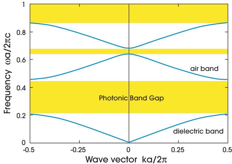
**Figure 5:** The photonic band structure of a multilayer film with lattice constant  $a$  and alternating layers of different widths. The width of the  $\varepsilon = 13$  layer is  $0.2a$ , and the width of the  $\varepsilon = 1$  layer is  $0.8a$ .
