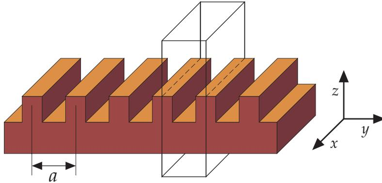
**Figure 5:** A dielectric configuration with discrete translational symmetry. If we imagine that the system continues forever in the  $y$  direction, then shifting the system by an integral multiple of  $a$  in the  $y$  direction leaves it unchanged. The repeated unit of this periodic system is framed with a box. This particular configuration is employed in distributed-feedback lasers, as in Yariv (1997).
