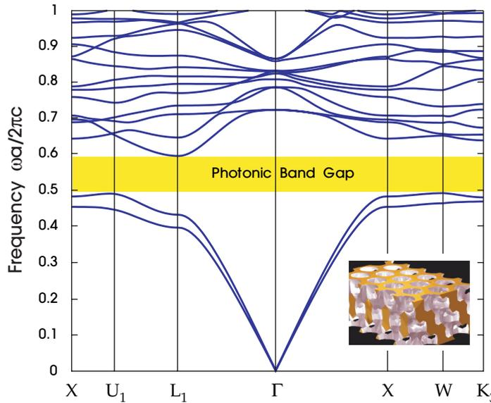
**Figure 5:** The photonic band structure for the lowest bands of Yablonovite (inset, from figure 4). Wave vectors are shown for a portion of the irreducible Brillouin zone that includes the edges of the complete gap (yellow). A detailed discussion of this band structure can be found in Yablonovitch et al. (1991a).
