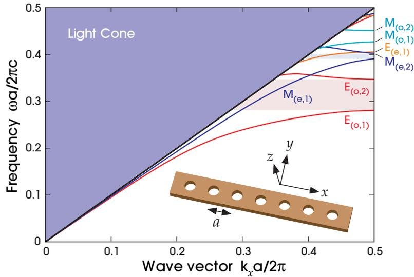
**Figure 5:** Band diagram for the waveguide of figure 1(a) (inset): a three-dimensional dielectric strip, suspended in air, with a period- $a$  sequence of cylindrical air holes. Only the irreducible Brillouin zone is shown. The discrete guided modes are labelled according to their symmetry as described in the text, with the fundamental  $E$  and  $M$  band gaps shaded light red and blue, respectively (the light cone is shaded darker blue, bounded by the light line in black).
