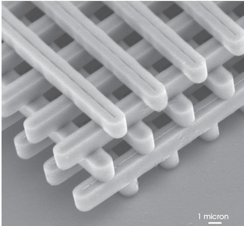
**Figure 6:** Electron-microscope image of a “woodpile” photonic crystal. The crystal is made of silicon and has a complete band gap centered at a wavelength of approximately 12 microns (Lin et al., 1998b). The dielectric “logs” form an fcc (or fct) lattice stacked in the [001] direction. (Image courtesy S.-Y. Lin.)
