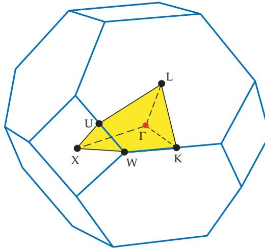
**Figure 4:** The Brillouin zone for the face-centered cubic (fcc) lattice. The reciprocal lattice is a body-centered cubic (bcc) lattice, and the Brillouin zone is a truncated octahedron with center at  $\Gamma$ . Also shown are some of the labels that are traditionally given to the special points in the zone. The irreducible Brillouin zone is the yellow polyhedron with corners at  $\Gamma$ , X, U, L, W, and K.
