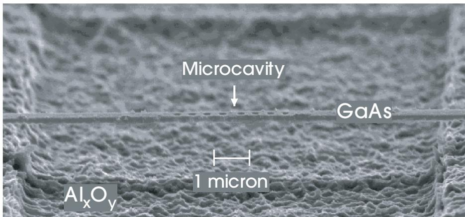
**Figure 8:** *Top:* Waveguide–cavity–waveguide filter formed in a suspended (“air bridge”) dielectric waveguide by a periodic sequence (period  $a$ ) of four air holes surrounding a defect (separation  $d > a$ ). *Middle:* Schematic diagram of this structure, similar to figure 5 but with the addition of a radiative lifetime  $\tau_r$ . *Bottom:* SEM image of fabricated structure in GaAs with period  $a \approx 0.5 \mu\text{m}$  (Ripin et al., 1999).
