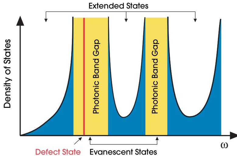
**Figure 12:** The division of frequency space into extended and evanescent states. In this sketch, the **density of states** (the number of allowed modes per unit frequency) is zero in the band gaps of the crystal (yellow). Modes are allowed to exist in these regions only if they are evanescent, and only if the translational symmetry is broken by a defect. Such a mode is shown in red.
