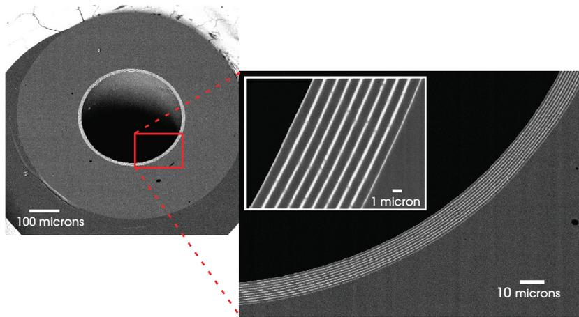
**Figure 13:** Electron-microscope image of a hollow-core omnidirectional-mirror Bragg-fiber cross section, with insets showing enlarged views of multilayer structures. Thin white layers are a chalcogenide glass and gray regions are a polymer. This fiber was designed to operate at a wavelength of  $10.6 \mu\text{m}$  (Temelkuran et al., 2002).
