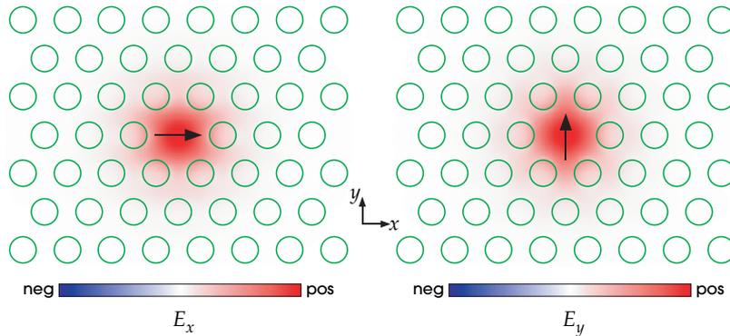
**Figure 3:** Electric-field pattern for the doubly degenerate fundamental mode of figure 2. Their polarizations are nearly orthogonal everywhere: the mode pictured at left is mostly  $E_x$ , and the mode pictured at right is mostly  $E_y$ . The green circles show the locations of the air holes.
