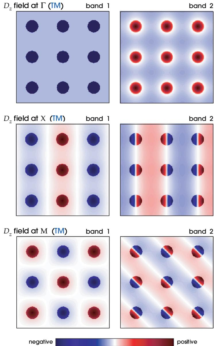
**Figure 3:** Displacement fields of TM states inside a square array of dielectric ( $\epsilon = 8.9$ ) columns in air. The color indicates the amplitude of the displacement field, which points in the  $z$  direction. Modes are shown at the  $\Gamma$  point (top), the X point (middle), and the M point (bottom). In each set, the dielectric band is on the left and the air band is on the right. The fields of the air band at the M point are from one of a pair of degenerate states.
