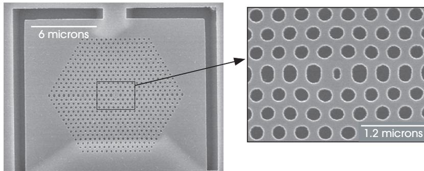
**Figure 17:** Electron-microscope image of experimental cavity structure in a hole-slab membrane (Lončar et al., 2002). Similar to the cavity of figure 16, but with reduced radius instead of increased  $\varepsilon$  for the central defect hole. (Image courtesy M. Lončar.)
