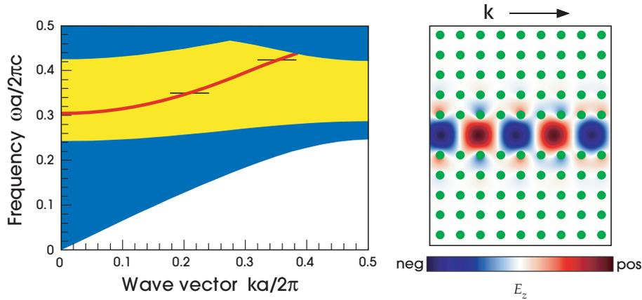
**Figure 2:** Line-defect waveguide formed by missing row of rods in square lattice of radius  $0.2a$  dielectric rods ( $\epsilon = 11.4$ ) in air. *Left:* projected band diagram, with extended modes of crystal shaded blue, TM gap shaded yellow, and guided mode (red line in gap). Horizontal black lines indicate low-dispersion range where guided band is nearly flat. *Right:* Electric field  $E_z$  of guided mode at  $\omega a / 2\pi c = 0.38$ , with dielectric rods in green.
