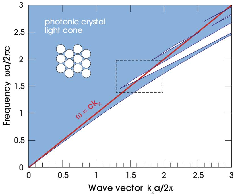
**Figure 7:** Projected band diagram, as a function of out-of-plane wave vector  $k_z$ , for a triangular lattice of air holes (inset: period  $a$ , radius  $0.47a$ ) in  $\epsilon = 2.1$ . This forms the light cone of the holey fiber from figure 1(b), with gaps appearing as open regions. The light line of air,  $\omega = ck_z$ , is shown in red. (Dashed box indicates region plotted in figures 10 and 12 for the defect modes.)
