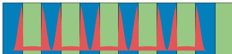
**Figure 4:** The modes associated with the lowest band gap that is shown in the band structure of the right-hand panel of figure 2, at  $k = \pi/a$ . The situation is similar to that of figure 3, but the dielectric contrast is larger. The blue and green regions correspond to  $\epsilon$  of 13 and 1, respectively.
