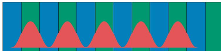
**Figure 3:** The modes associated with the lowest band gap of the band structure plotted in the center panel of figure 2, at  $k = \pi/a$ . (a) Electric field of band 1; (b) electric field of band 2; (c) electric-field energy density  $\epsilon |\mathbf{E}|^2/8\pi$  of band 1; (d) electric-field energy density of band 2. In the depiction of the multilayer film, blue indicates the region of *higher* dielectric constant ( $\epsilon = 13$ ).
