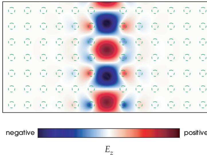
**Figure 18:** Electric-field ( $E_z$ ) pattern associated with a linear defect formed by removing a column of rods from an otherwise-perfect square lattice of rods in air. The resulting field, shown here for a wave vector  $k_y = 0.3(2\pi/a)$  along the defect, is a **waveguide mode** propagating along the defect. The rods are shown as dashed green outlines.
