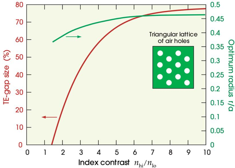
**Figure 7:** Gap recipe for the lowest TE gap of the triangular lattice of air holes in dielectric.
