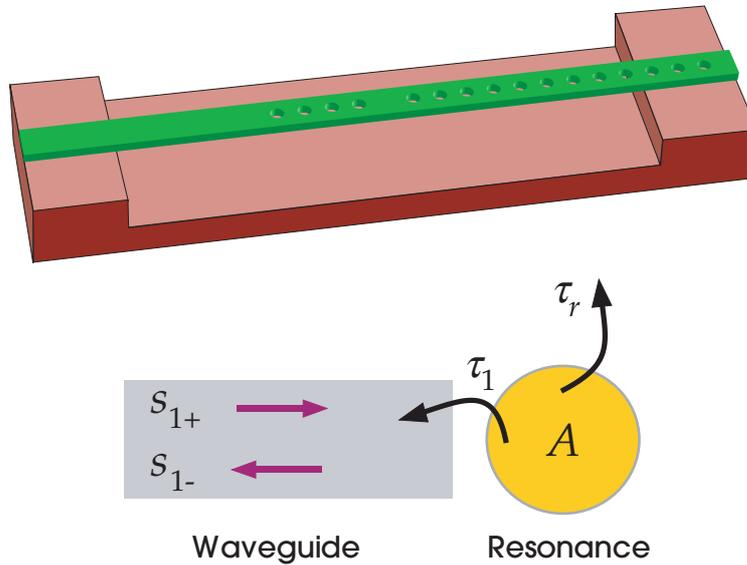
**Figure 10:** Schematic of air-bridge structure designed to radiate rather than transmit light on resonance: transmission is blocked by the band gap of many periods of holes on the right side of the cavity. This is modelled abstractly (bottom), similar to figure 5, by a resonant cavity coupled only to a single input waveguide and to radiation, but no output waveguide. The result is that  $\tau_1 = \tau_r$  in order to maximize radiation on resonance, ideally achieving 100% radiation.
