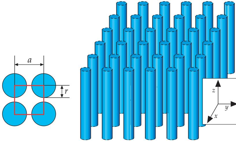
**Figure 1:** A two-dimensional photonic crystal. This material is a square lattice of dielectric columns, with radius  $r$  and dielectric constant  $\epsilon$ . The material is homogeneous along the  $z$  direction (we imagine the cylinders are very tall), and periodic along  $x$  and  $y$  with lattice constant  $a$ . The left inset shows the square lattice from above, with the unit cell framed in red.
