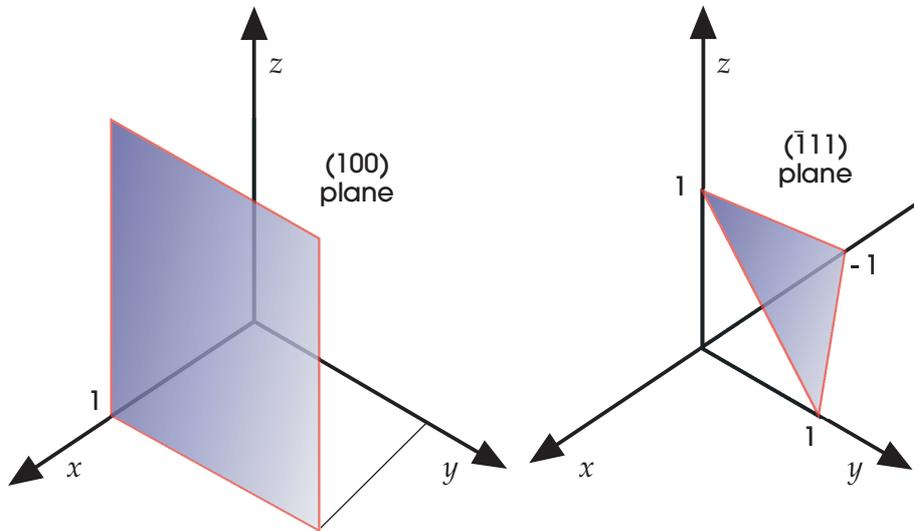
**Figure 6:** Special cases of the Miller index system. *Left:* The (100) plane of a simple-cubic lattice. The plane never intersects the  $y$  or  $z$  axes, so the corresponding indices are zero. *Right:* The  $(\bar{1}11)$  plane of the simple-cubic lattice. The plane intersects the  $x$  axis at  $-1$ , so a bar is placed over the corresponding index.
