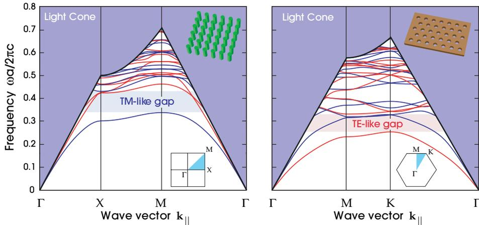
**Figure 2:** Band diagrams for photonic crystal slabs of figure 1, suspended in air (inset): the **rod slab** (left) and the **hole slab** (right). The blue shaded area is the *light cone*, all of the extended modes propagating in air. Below it are the guided bands localized to the slab: blue/red bands indicate TM/TE-like modes, respectively (odd/even with respect to the  $z = 0$  mirror plane). The rod/hole slabs have gaps in the TM/TE-like modes, which are shaded light blue/red respectively.
