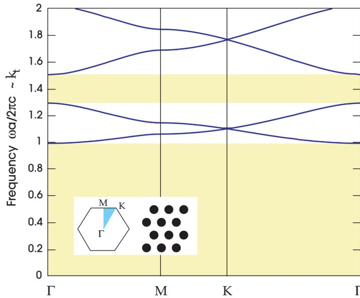
**Figure 5:** Band diagram for TM-polarized modes of a two-dimensional triangular lattice of perfect-metal cylinders. Two band gaps are shown (shaded yellow), where the lowest band has a low-frequency cutoff characteristic of metallic structures. These bands are equivalent to the modes of the holey fiber in the scalar (large  $k_z$ ) limit.
