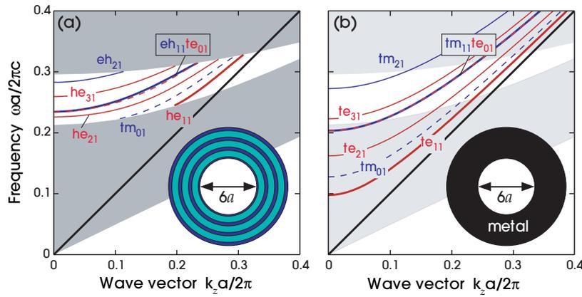
**Figure 15:** (a) Band diagram of hollow-core ( $R = 3a$ ) Bragg fiber with layer indices of 2.7/1.6 (blue/green layers in inset); gray regions indicate extended modes that propagate in the multilayer mirrors. (b) Band diagram showing the first few bands of a hollow perfect-metal waveguide of the same radius; light gray regions indicate extended modes of Bragg mirrors from (a), for comparison. Modes are labelled by polarization and radial/angular mode numbers as described in the text.
