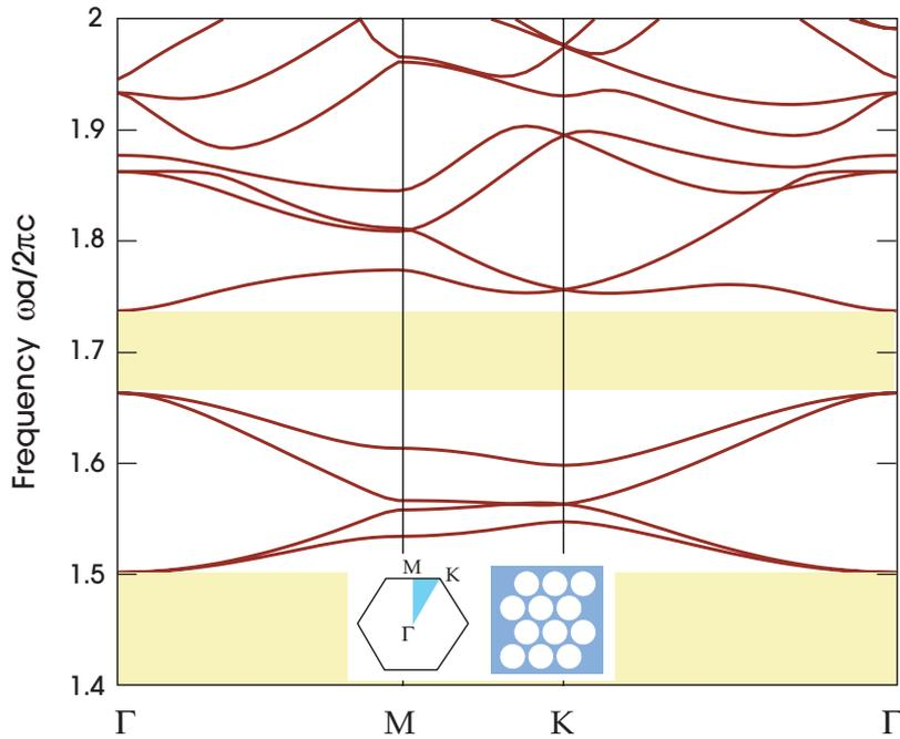
**Figure 8:** Band diagram versus in-plane wave vector in the irreducible Brillouin zone (inset) for the triangular lattice of air holes from figure 7, at an out-of-plane wave vector  $k_z a/2\pi = 1.7$ . Gaps are shaded yellow: the lower gap corresponds to the index-guiding region, and the upper gap corresponds to one of the band gaps inside the light cone where guiding in an air core is possible.
