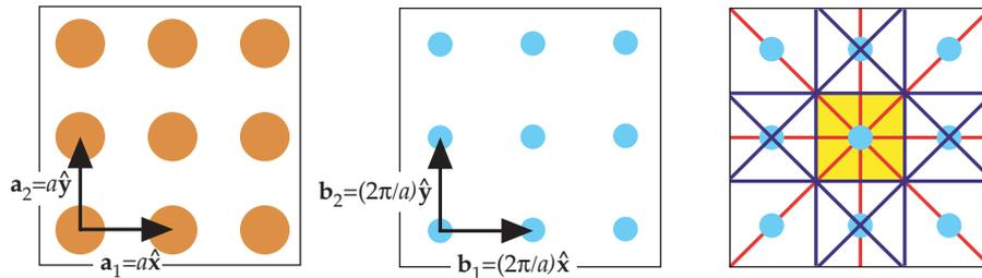
**Figure 2:** The square lattice. On the left is the network of lattice points in real space. In the middle is the corresponding reciprocal lattice. On the right is the construction of the first Brillouin zone: taking the center point as the origin, we draw the lines connecting the origin to the other lattice points (red), their perpendicular bisectors (blue), and highlight the square boundary of the Brillouin zone (yellow).
