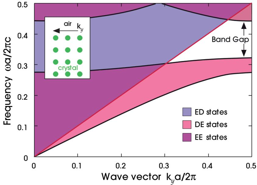
**Figure 20:** The projected band structure of the constant- $x$  surface of the square lattice of alumina rods in air. The shading denotes regions in which light is transmitted (purple  $EE$  states), internally reflected (red  $DE$  states), and externally reflected (blue  $ED$  states). The crystal is terminated as shown in the inset; this termination has no surface states.
