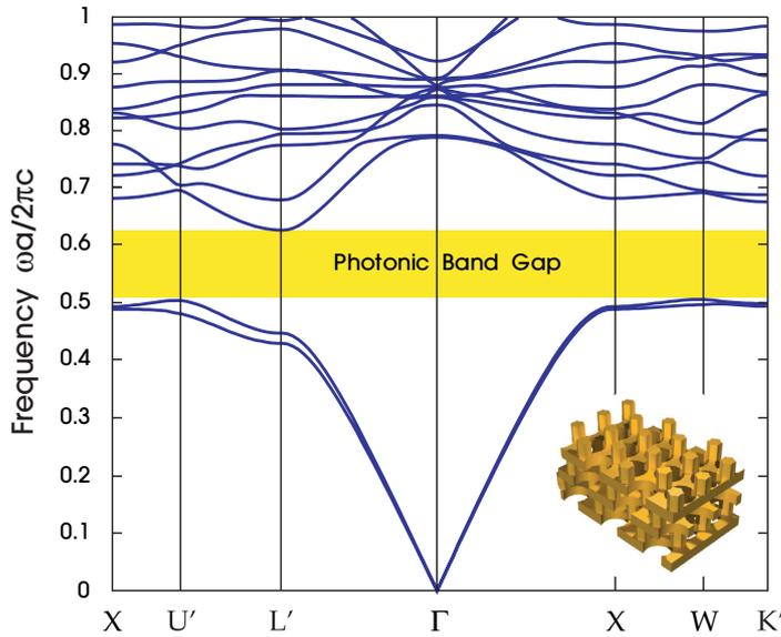
**Figure 11:** The photonic band structure for the lowest bands of the layered structure from figure 10 (inset). The irreducible Brillouin zone is larger than that of the fcc lattice described in appendix B, because of reduced symmetry—only a portion is shown, including the edges of the complete photonic band gap (yellow). A more detailed discussion of this band structure can be found in Johnson and Joannopoulos (2000).
