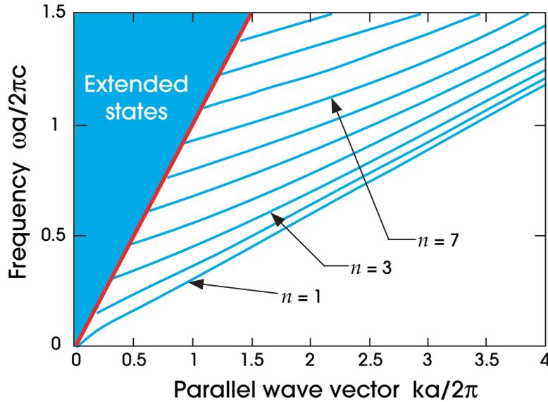
**Figure 3:** Harmonic mode frequencies for a plane of glass of thickness  $a$  and  $\epsilon = 11.4$ . Blue lines correspond to modes that are localized in the glass. The shaded blue region is a continuum of states that extend into both the glass and the air around it. The red line is the **light line**  $\omega = ck$ . This plot shows modes of only one polarization, for which  $\mathbf{H}$  is perpendicular to both the  $z$  and  $k$  directions.
