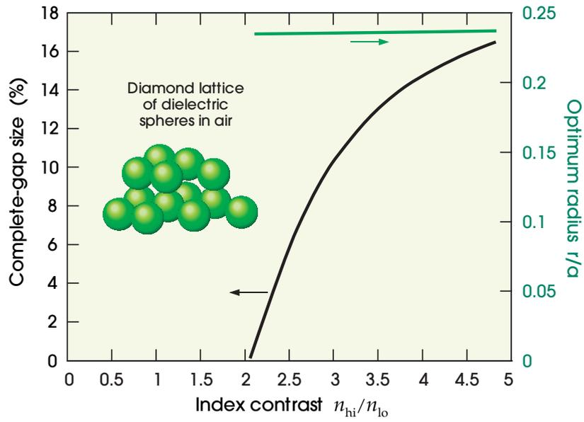
**Figure 10:** Gap recipe for the lowest *complete* gap of the diamond lattice of dielectric spheres in air.
