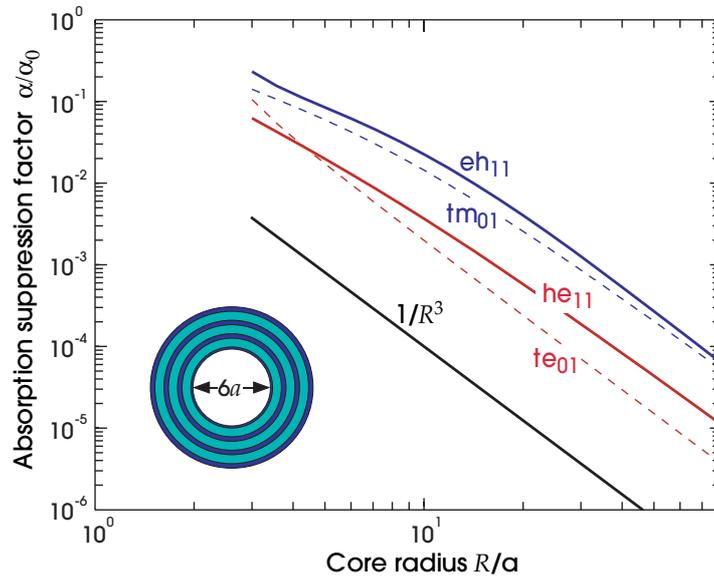
**Figure 18:** Scaling of the absorption suppression factor  $\alpha/\alpha_0$  versus core radius  $R$ , at quarter-wave frequency, for several modes of the hollow-core Bragg fiber with indices 2.7/1.6 (blue/green in inset). The absorption loss is assumed to be dominated by that of the low-index material. All modes asymptote to a  $1/R^3$  scaling (shown as a black line, for reference).
