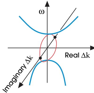
**Figure 6:** Schematic illustration of the complex band structure of the multilayer film. The upper and lower blue lines correspond to the bottom of band 2 and the top of band 1, respectively. The evanescent states occur on the red line, which extends along the imaginary- $k$  axis running out of the page. The maximum decay occurs roughly at the center of the gap.
