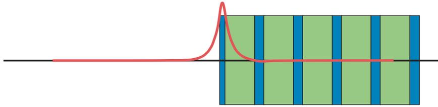
**Figure 13:** The electric field strength associated with a localized mode at the surface of a multilayer film. In particular, the mode at  $k_y = 2\pi/a$  from figure 14 is shown. (This mode actually oscillates in sign with each period of the crystal, but with an amplitude too small to see clearly here.)
