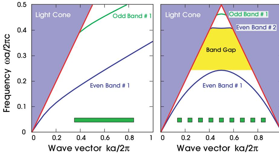
**Figure 3:** Band diagrams of waveguides from figure 2, for TM-polarized in-plane ( $k_z = 0$ ) light only. *Left:* uniform waveguide of figure 2(a). *Right:* periodic waveguide of figure 2(b), including twice the irreducible Brillouin zone. Blue shaded region is light cone (extended states propagating in air). Discrete guided bands are labelled even or odd according to the  $y = 0$  mirror symmetry plane.
