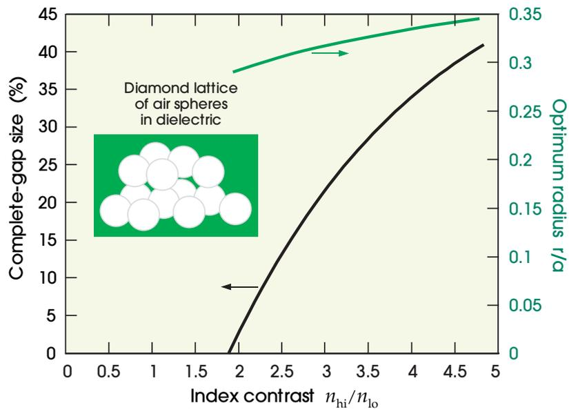
**Figure 11:** Gap recipe for the lowest *complete* gap of the diamond lattice of spherical air holes in dielectric.
