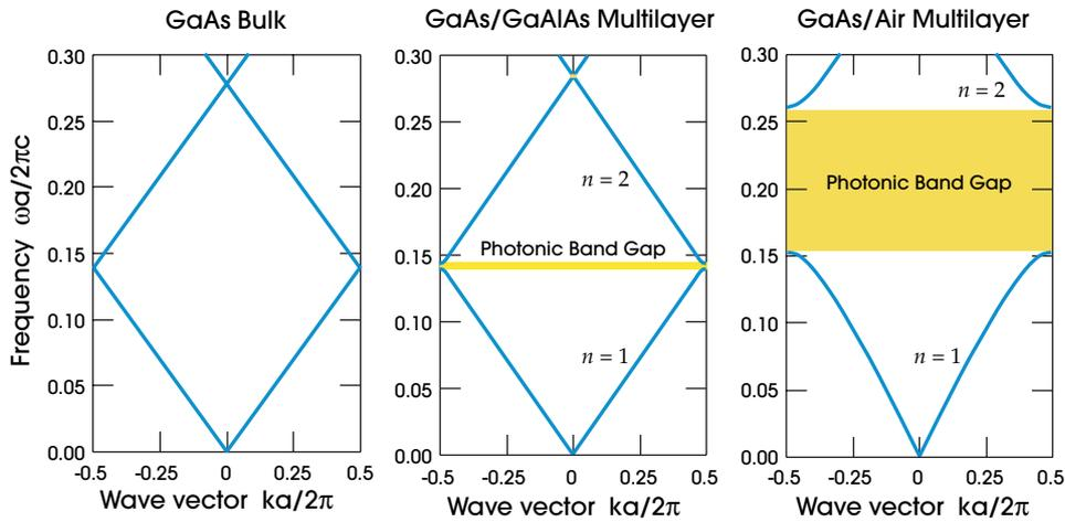
**Figure 2:** The photonic band structures for on-axis propagation, as computed for three different multilayer films. In all three cases, each layer has a width  $0.5a$ . *Left:* every layer has the same dielectric constant  $\epsilon = 13$ . *Center:* layers alternate between  $\epsilon$  of 13 and 12. *Right:* layers alternate between  $\epsilon$  of 13 and 1.
