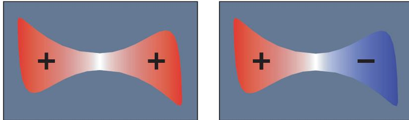
**Figure 1:** A two-dimensional metallic cavity with inversion symmetry. Red and blue suggest positive and negative fields. On the left, an **even** mode occupies the cavity, for which  $\mathbf{H}(\mathbf{r}) = \mathbf{H}(-\mathbf{r})$ . On the right, an **odd** mode occupies the cavity, for which  $\mathbf{H}(\mathbf{r}) = -\mathbf{H}(-\mathbf{r})$ .
