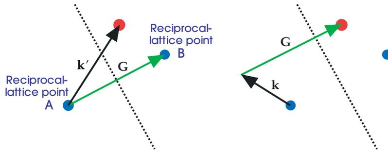
**Figure 1:** Characterization of the Brillouin zone. The dotted line is the perpendicular bisector of the line joining two reciprocal lattice points (blue). If we choose the left point as the origin, any lattice vector (such as  $\mathbf{k}'$ ) that reaches to an arbitrary point on the other side (red) can be expressed as the sum of a same-side vector (such as  $\mathbf{k}$ ) plus a reciprocal lattice vector  $\mathbf{G}$ .
