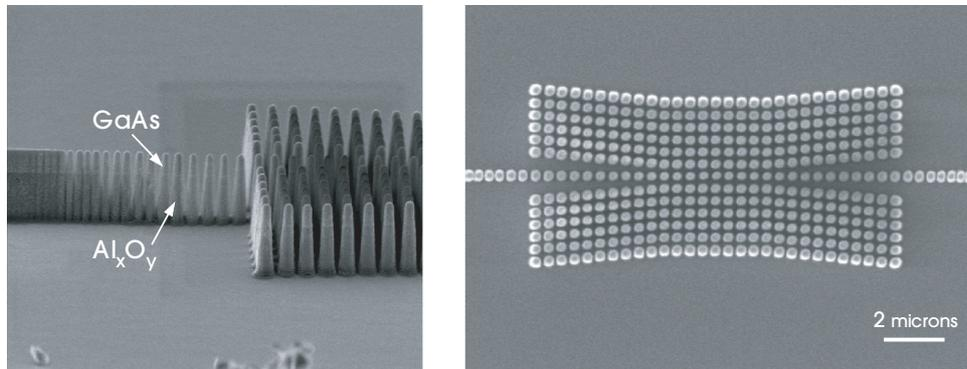
**Figure 4:** Two views of a reduced-radius waveguide fabricated in a rod slab by Assefa et al. (2004), designed to operate at near-infrared wavelengths. (GaAs rods on low-index aluminum-oxide pedestals.) The structure was designed to couple the reduced-radius waveguide via an adiabatic taper to a dielectric strip waveguide at the ends. (Images courtesy L. Kolodziejski.)
