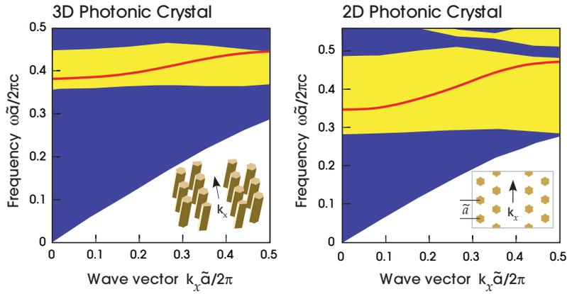
**Figure 18:** *Left:* Projected band diagram of the line defect from figure 17, formed by a missing row of rods from a single layer of the three-dimensional crystal from figure 10. The red line is the guided band in the complete photonic band gap (yellow). Inset shows a single rod layer with the defect (other layers of the crystal not shown). *Right:* Projected band diagram of TM states for the corresponding two-dimensional crystal with an identical rod cross section (inset).
