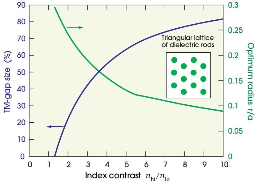
**Figure 5:** Gap recipe for the lowest TM gap of the triangular lattice of dielectric rods.
