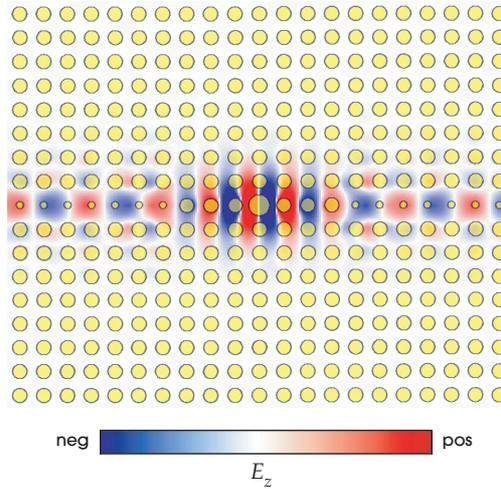
**Figure 12:** Waveguide–cavity–waveguide filter in square lattice of rods, similar to figure 4 but with slightly different parameters. Crystal:  $\epsilon = 5.4$  rods with radius  $r = 0.2a$  and an 18% TM gap. Waveguide: row of reduced-radius ( $r = 0.08a$ ) rods. Cavity: increased-radius ( $r = 0.42a$ ) rod with a dipole-like state at  $\omega_0 a/2 \pi c = 0.25814$ .
