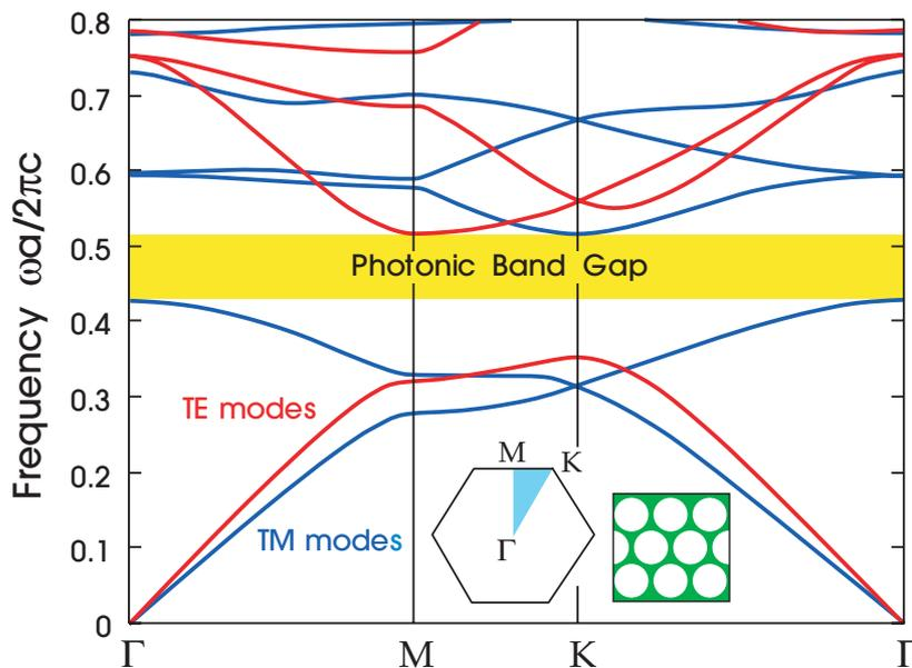
**Figure 10:** The photonic band structure for the modes of a triangular array of air columns drilled in a dielectric substrate ( $\epsilon = 13$ ). The blue lines represent TM bands and the red lines represent TE bands. The inset shows the high-symmetry points at the corners of the irreducible Brillouin zone (shaded light blue). Note the complete photonic band gap.
