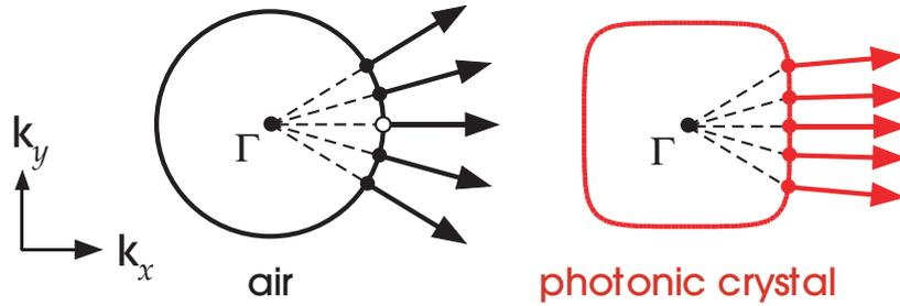
**Figure 16:** Isofrequency contours in air (left, black) and in the photonic crystal (right, red) of figure 15 (the  $\omega a/2\pi c = 0.496$  contour of the second band). Arrows show the group velocity directions for a variety of  $\mathbf{k}$  vectors (dots) with different  $k_y$  components. The nearly flat contour of the photonic crystal means that a finite-width beam made up of these wave vectors will spread (diffract) very slowly compared to air, an effect called *supercollimation*.
