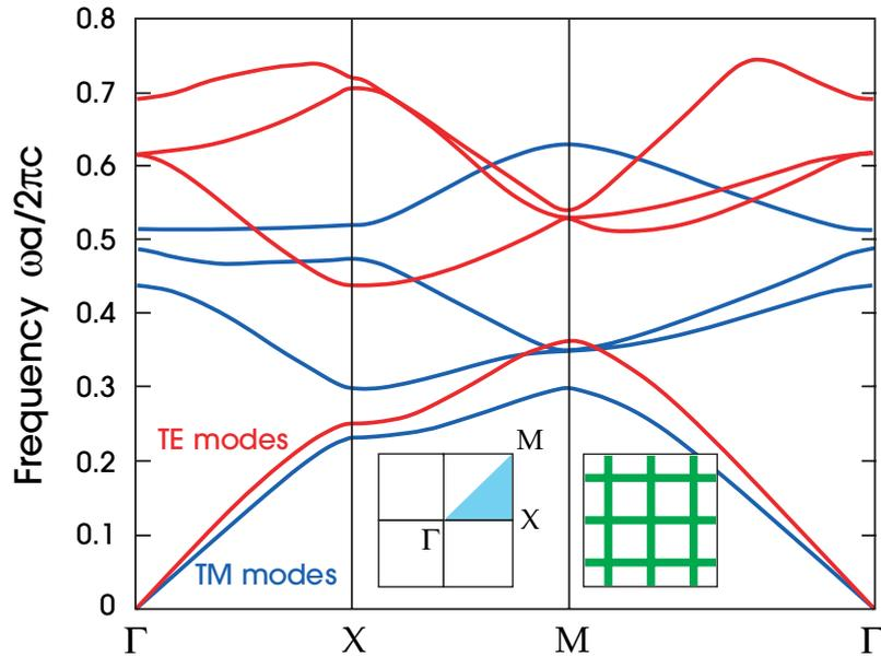
**Figure 5:** The photonic band structure for the lowest-frequency modes of a square array of dielectric ( $\epsilon = 8.9$ ) veins (thickness  $0.165a$ ) in air. The blue lines are TM bands and the red lines are TE bands. The left inset shows the high-symmetry points at the corners of the irreducible Brillouin zone (shaded light blue). The right inset shows a cross-sectional view of the dielectric function.
