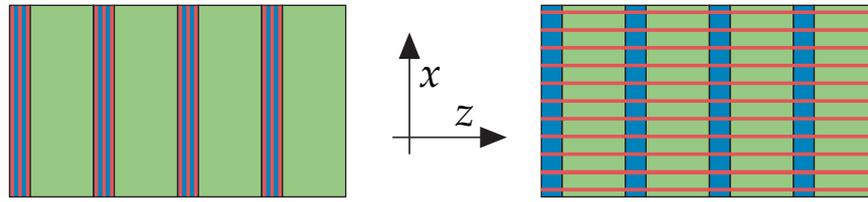
**Figure 9:** A sketch of the displacement field lines for a long-wavelength mode traveling in the  $y$  direction (out of the page). In the left figure, the fields are oriented along  $x$ . In the right figure, the fields are oriented primarily along  $z$ . The blue regions correspond to high  $\epsilon$ .
