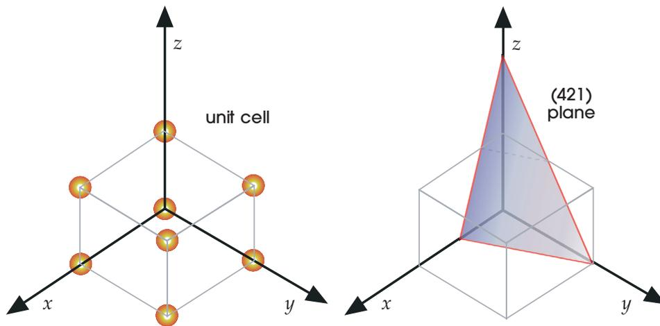
**Figure 5:** The Miller indices for a crystal plane. *Left:* A plot of the unit cell. The length of the unit cell in each direction is the lattice constant for that direction. *Right:* The shaded plane is named by locating the intercepts of the plane with the axes, as described in the text.
