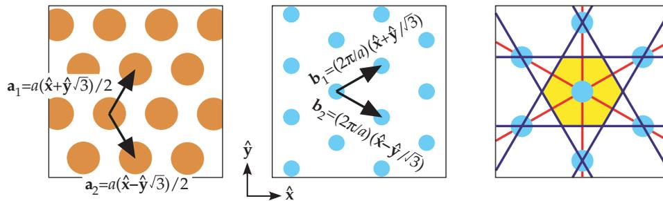
**Figure 3:** The triangular lattice. On the left is the network of lattice points in real space. In the middle is the corresponding reciprocal lattice, which in this case is a rotated version of the original. On the right is the Brillouin zone construction. In this case, the first Brillouin zone is a hexagon centered around the origin.
