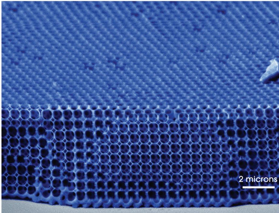
**Figure 9:** Electron-microscope image (artificial coloring) of inverse-opal structure demonstrated to have a complete band gap around a wavelength of 1.3 microns in Vlasov et al. (2001). Unlike figure 8, this is actually an fcc lattice of hollow dielectric (silicon) *shells*, which increases the size of the gap. (Image courtesy D. J. Norris.)
