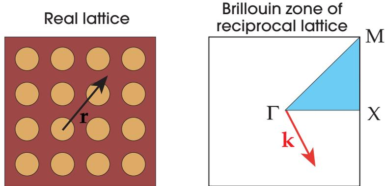
**Figure 6:** *Left:* A photonic crystal made using a square lattice. An arbitrary vector  $\mathbf{r}$  is shown. *Right:* The Brillouin zone of the square lattice, centered at the origin ( $\Gamma$ ). An arbitrary wave vector  $\mathbf{k}$  is shown. The **irreducible zone** is the light blue triangular wedge. The special points at the center, corner, and face are conventionally known as  $\Gamma$ ,  $M$ , and  $X$ .
