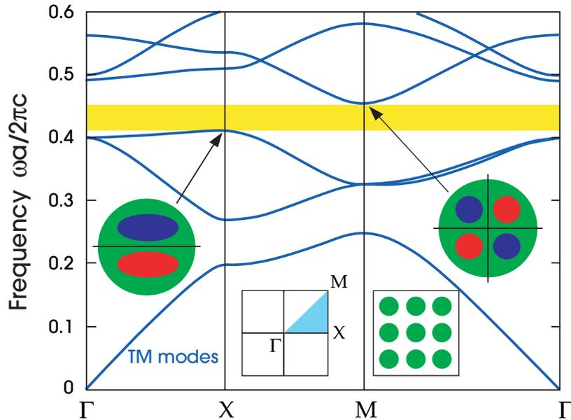
**Figure 13:** The TM modes of a square array of dielectric ( $\epsilon = 8.9$ ) columns in air, with  $r = 0.38a$ . The center inset shows the irreducible Brillouin zone (shaded light blue). The other two insets suggest the field patterns of the modes, within each column (red/blue for positive/negative fields). The left inset shows the  $\pi$ -like pattern for band 3; the right shows the  $\delta$ -like pattern for the bottom of band 4.
