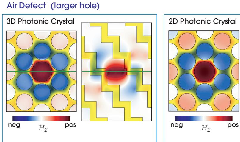
**Figure 15:** Horizontal and vertical cross sections (intersecting at green lines) of  $H_z$  field patterns of point defects in the layered structure from figure 10 (left), formed by modifying increasing the radius of a single hole in a hole layer, compared to the field for the corresponding TE state in a two-dimensional crystal (right) with the same *hole* cross section. Dielectric material is shown in yellow.
