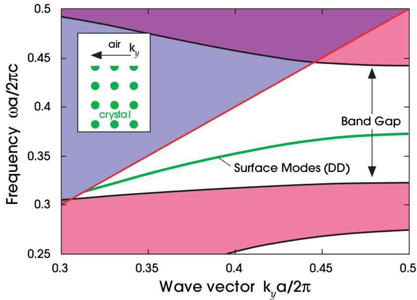
**Figure 21:** The projected band structure of the constant- $x$  surface of the square lattice of alumina rods in air, like figure 20 above except with a different termination shown in the inset. The line in the gap corresponds to a surface band in which light is exponentially localized to the surface (green,  $DD$ ).
