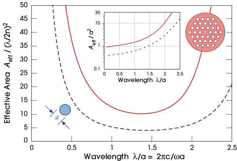
**Figure 6:** Effective area, in units of the wavelength squared, as a function of wavelength, for the solid-core holey fiber with period  $a$  (solid red line) and a simple dielectric cylinder of diameter  $a$  (dashed blue line). Inset is the same plot, but with the effective area in units of  $a^2$ .
