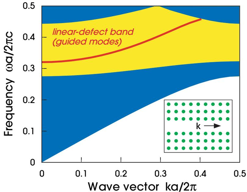
**Figure 19:** The projected band structure of the line defect (inset) formed by removing a row (or column) of rods from an otherwise perfect square lattice from figure 2, plotted versus the wave vector component  $k$  along the defect. The extended modes in the crystal become continuum regions (blue), whereas inside the band gap (yellow) a defect band (red) is introduced corresponding to a localized state as in figure 18.
