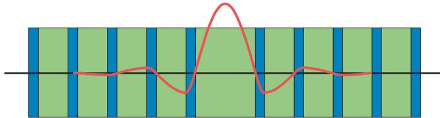
**Figure 11:** A defect in a multilayer film, formed by doubling the thickness of a single *low- $\epsilon$*  layer in the structure of figure 5. Note that this can be considered to be an interface between two perfect multilayer films. The red curve is the electric-field strength of the defect state associated with this structure (for on-axis propagation).
