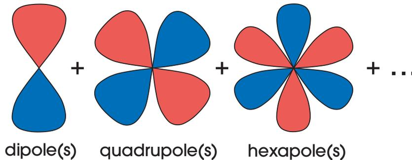
**Figure 14:** Schematic depiction of multipole expansion: the field radiated by a localized source is expanded as a sum of dipole, quadrupole, et cetera contributions, corresponding to an expansion in spherical harmonics. There are generally several terms of each type (e.g. dipoles oriented in different directions).
