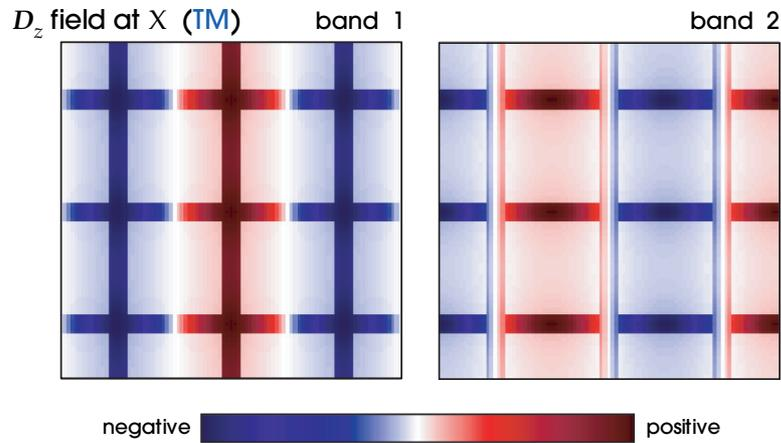
**Figure 6:** Displacement fields of X-point TM modes for a square array of dielectric ( $\epsilon = 8.9$ ) veins in air. The color indicates the amplitude of the displacement field, which is oriented in the  $z$  direction (out of the page). The dielectric band is on the left, and the air band is on the right.
