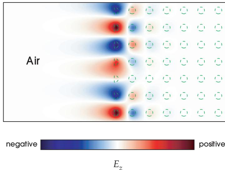
**Figure 22:** Electric-field ( $E_z$ ) pattern associated with a surface-localized state formed by truncating a square lattice of alumina rods in air, cutting each rod in half at the boundary as in figure 21. The mode shown corresponds to a surface-parallel wave vector  $k_y = 0.4(2\pi/a)$ . The dielectric rods are shown as dashed green outlines.
