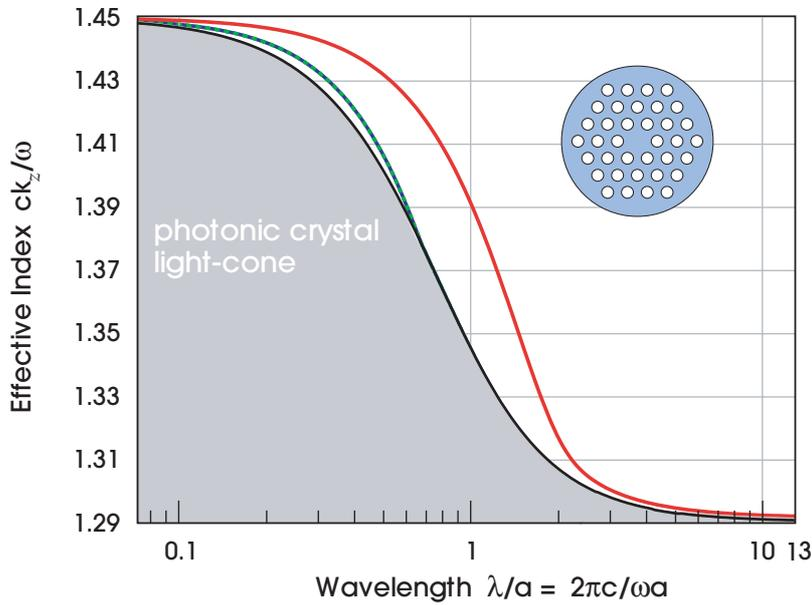
**Figure 4:** Bands of the solid-core holey fiber, from figure 2, plotted as “effective index”  $ck_z/\omega$  versus wavelength, along with the light cone (gray region). In the limit of small  $\lambda$ , the effective indices of both the modes and the light line approach the index 1.45 of the bulk silica.
