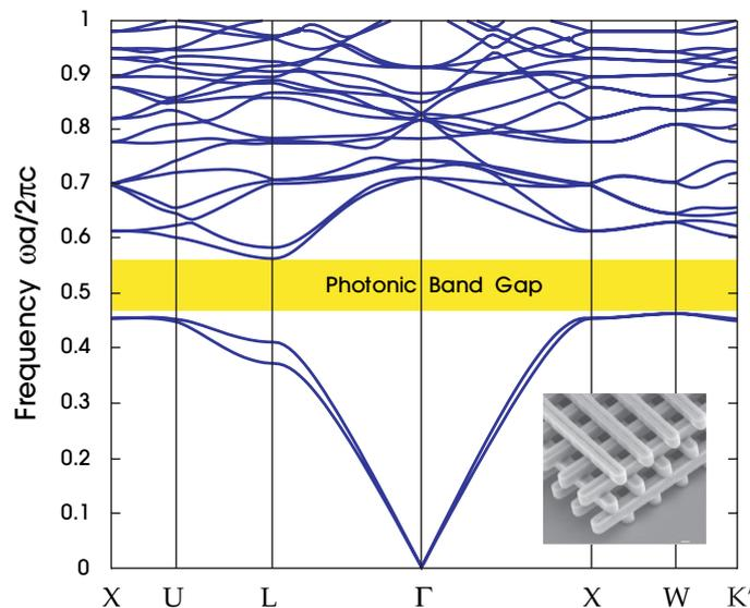
**Figure 7:** The photonic band structure for the lowest bands of the woodpile structure (inset, from figure 6) with  $\epsilon = 13$  logs in air. The irreducible Brillouin zone is larger than that of the fcc lattice described in appendix B, because of reduced symmetry—only a portion is shown, including the edges of the complete photonic band gap (yellow).
