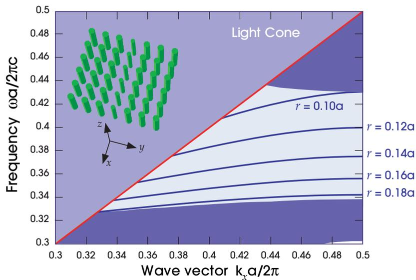
**Figure 5:** Projected band diagram of TM-like ( $z$ -odd) states in a linear waveguide in the rod slab of figure 2(left), formed by reducing the radius of a row of rods (inset), as a function of the wave vector  $k_x$  along the defect. The dark blue shaded regions below the light line are extended modes in the crystal. The rods in the bulk crystal have radius  $r = 0.2a$ ; the localized waveguide bands for five different defect radii are labelled in the gap.
