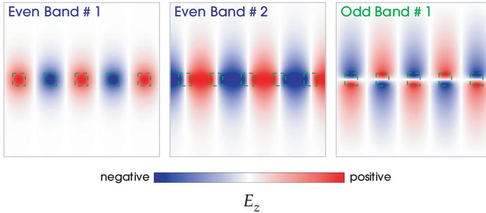
**Figure 4:**  $E_z$  field patterns of the periodic waveguide from figure 2(b) at  $k = \pi/a$ , the Brillouin-zone edge, labelled as in figure 3. Left and middle panels correspond to the edges of the gap in the even guided modes, while the right panel has odd symmetry with respect to the  $y = 0$  mirror plane. The dielectric squares are shown as dashed green lines.
