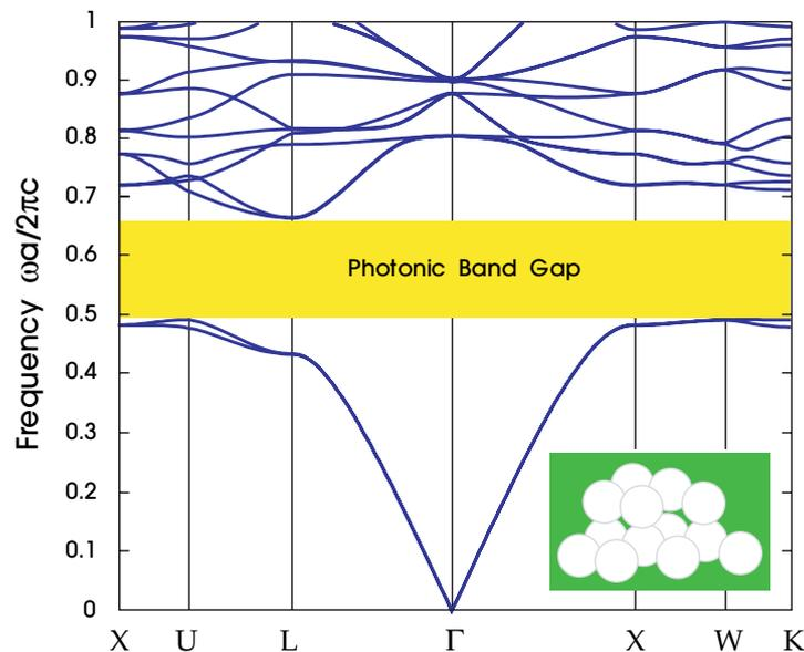
**Figure 3:** The photonic band structure for the lowest bands of a diamond lattice of air spheres in a high dielectric ( $\epsilon = 13$ ) material (inset). A complete photonic band gap is shown in yellow. The wave vector varies across the irreducible Brillouin zone between the labelled high-symmetry points; see appendix B for a discussion of the Brillouin zone of an fcc lattice.
