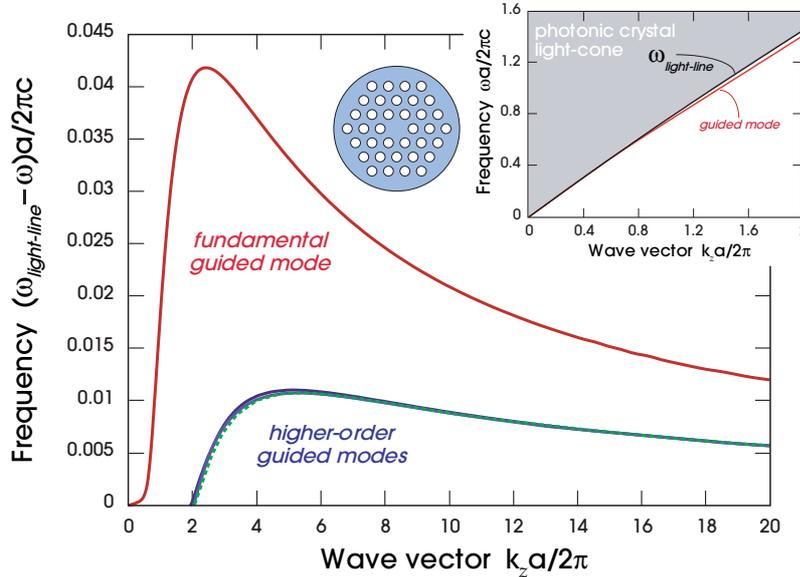
**Figure 2:** Band diagram of solid-core holey fiber as a function of axial wave vector  $k_z$ . The usual  $\omega$  plot is inset, but for clarity we also plot the  $\Delta\omega$  between the guided bands and the light line. The higher-order guided modes are three bands that are nearly on top of one another.
