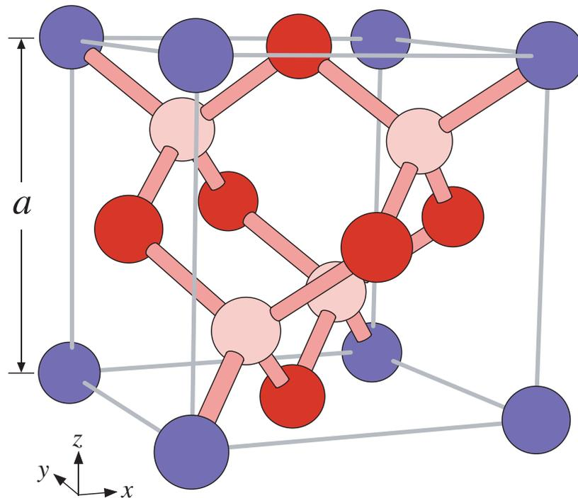
**Figure 1:** Ball-and-stick (“atomic”) representation of several three-dimensional lattices in a cubic supercell, with a lattice constant  $a$ . The blue balls alone form a simple cubic lattice. Adding the dark red balls produces a face-centered cubic (fcc) lattice. Adding the pink balls as well produces a diamond lattice, with stick “bonds” (four bonds per ball).
