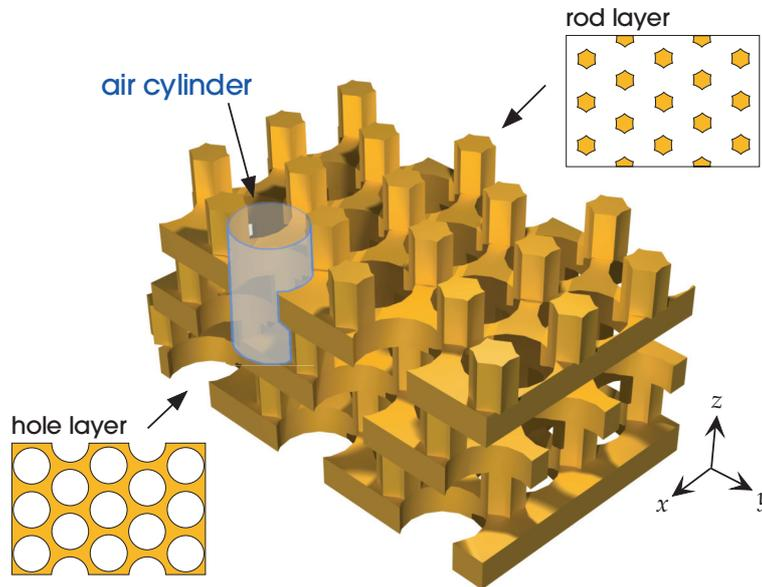
**Figure 10:** Three-dimensional photonic crystal formed by a stack of layers with two-dimensional cross sections: triangular lattices of dielectric rods in air (upper-right inset) and holes in dielectric (lower-left inset). These layers are paired in bilayers with an  $ABCABC \dots$  stacking, and are formed from a face-centered cubic (fcc) lattice of overlapping air cylinders in dielectric (one is highlighted) oriented along the  $[111]$  direction.
