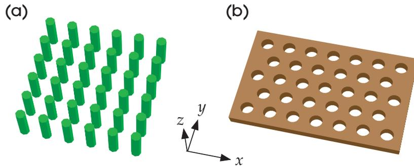
**Figure 1:** Examples of **photonic-crystal slabs**, which combine two-dimensional periodicity (in the  $xy$  directions) and index-guiding in the vertical ( $z$ ) direction. (a) The **rod slab**, a square lattice of dielectric rods in air. (b) The **hole slab**, a triangular lattice of air holes in a dielectric slab.
