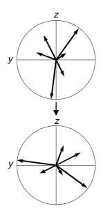
Each spin makes a contribution to the magnetization in each direction (top diagram). A pulse, here 90° about the *x*axis, rotates all of these contributions in the same sense through the same angle (bottom diagram).
