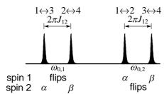
The spectrum from two coupled spins, showing which spins are passive and active in each transition. The frequency scale is in rad s<sup>-1</sup>, so the splitting of the doublet is  $2\pi J_{12}$  rad s<sup>-1</sup>, which corresponds to  $J_{12}$  Hz.
