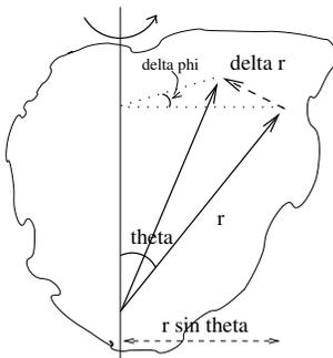
Figure 3: Infinitesimal displacement due to a rotation
