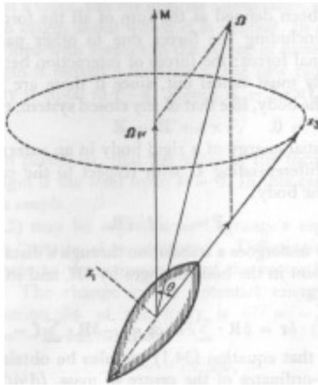
Figure 4: Fig 46 of symmetric top from Landau & Lifshitz.  $\mathbf{M} = \mathbf{L}$  is vertical and axis is along  $\hat{x}_3 = \hat{z}$ . The  $x_1$  principal axis has been marked, and chosen to lie in the plane of the axis of the top and the angular momentum vector. It is not fixed in the body, if the body spins on its axis.
