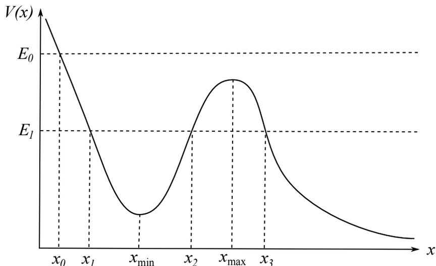
Figure 9: A general potential  $V(x)$ , with various points marked on the  $x$  axis.  $x_{\min}$  and  $x_{\max}$  are a local minimum and local maximum, respectively. At any point  $x$  the force acting on the particle is *minus the slope of the potential*,  $F(x) = -V'(x)$ .
