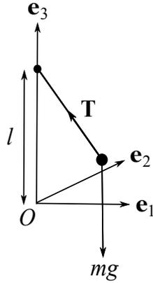
Figure 33: Foucault's pendulum. The position of the mass  $m$  is  $\mathbf{r} = (x, y, z) = x \mathbf{e}_1 + y \mathbf{e}_2 + z \mathbf{e}_3$ , with coordinates constrained via  $x^2 + y^2 + (l - z)^2 = l^2$ .
