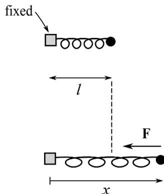
Figure 5: A spring lying along the  $x$  axis, with one end fixed at the origin. The first diagram shows the equilibrium position, while the second shows the spring extended by a length  $x - l > 0$ , with the resulting restoring force. Notice that when  $x - l < 0$ , which compresses the spring rather than stretches it, the force acts in the opposite direction (to the right).
