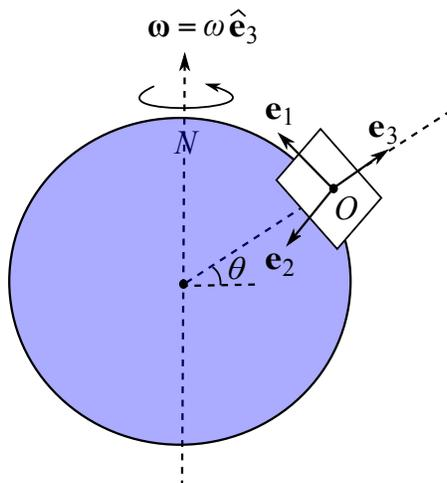
Figure 32: A frame  $\mathcal{S}$  fixed to the surface of the rotating Earth. The angular velocity  $\omega = 2\pi$  radians per day, or  $\omega \simeq 7 \times 10^{-5} \text{ s}^{-1}$ . The latitude of the origin  $O$  of  $\mathcal{S}$  is  $\theta$ .
