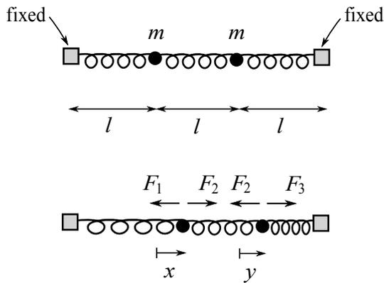
Figure 12: The system of masses and springs. The upper diagram shows the equilibrium configuration. In the lower diagram we have shown the horizontal displacements  $x$  and  $y$  of the two masses from their equilibrium positions, together with the various Hooke's law forces  $F_1$ ,  $F_2$ ,  $F_3$  acting.
