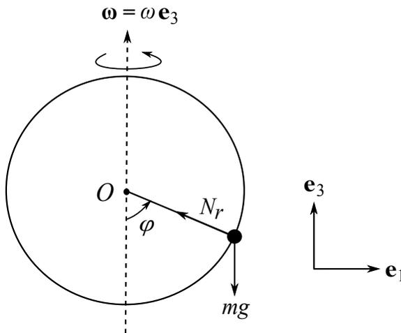
Figure 31: The bead on the rotating hoop. Here the figure shows the hoop at the instant at which it passes through the plane of the page. The component  $N_2$  of the normal reaction  $\mathbf{N}$  of the hoop on the bead points into the page at this instant, which is the  $\mathbf{e}_2$  direction.
