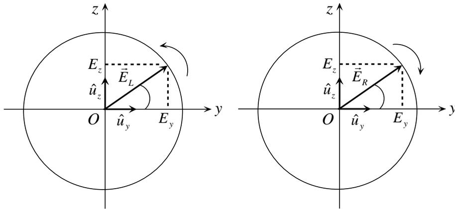
Fig. 10.14. Left-handed and right-handed polarized e/m wave.
