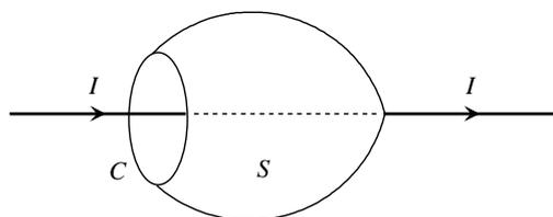
Fig. B.1. A loop  $C$  encircling the current  $I$ ; the open surface  $S$  is bordered by  $C$ .
