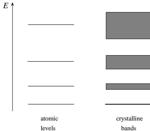
Fig. 1.7. Atomic energy levels (left) and the corresponding crystalline bands (right).
