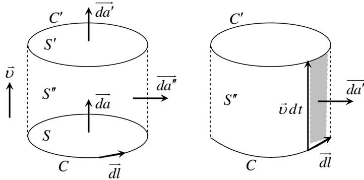
Fig. 9.8. A closed plane wire moving inside a static magnetic field.
