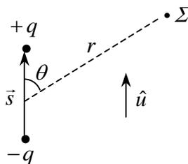
Fig. 10.10. An electric dipole a distance  $r$  from the observation point  $\Sigma$ .
