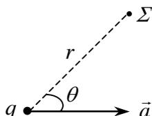
Fig. 10.8. An accelerating charge  $q$  a distance  $r$  from the observation point  $\Sigma$ .
