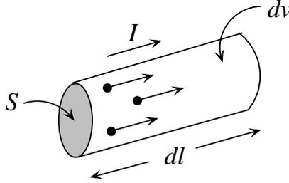
Fig. 2.5. Metal wire of infinitesimal length  $dl$ , carrying a current  $I$ .
