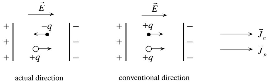
Fig. 2.7. Current densities of electrons and holes: actual and conventional directions of motion of charges.
