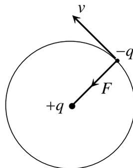
Fig. 1.1. Rutherford’s picture of the hydrogen atom.
