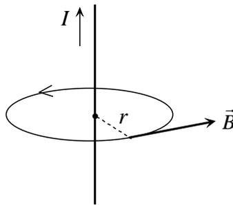
Fig. 7.6. Magnetic field line around a rectilinear current  $I$ .
