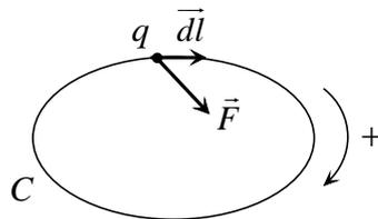
Fig. 9.1. Force on a test charge  $q$  at a point of an oriented loop  $C$ .
