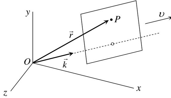
Fig. 10.4. Wave surface of a plane wave traveling in an arbitrary direction.
