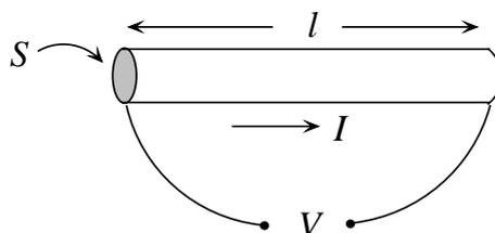
Fig. 2.6. Metal wire of finite length  $l$ , carrying a current  $I$  and subject to a voltage  $V$ .
