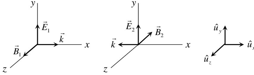
Fig. 10.6. Two monochromatic e/m waves traveling in opposite directions along the  $x$ -axis.
