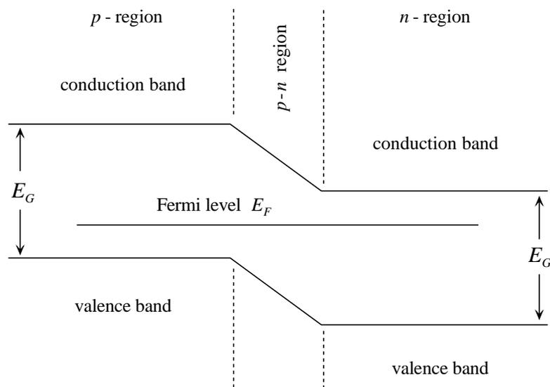
Fig. 3.7. Fermi level in a *p-n* junction.
