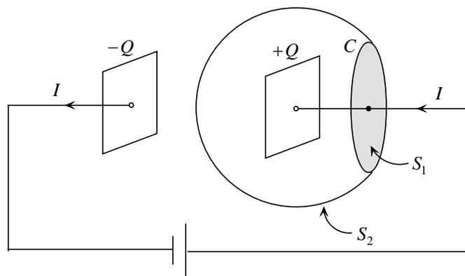
Fig. B.2. A flat surface  $S_1$  and a curved surface  $S_2$  with common border  $C$ . Part of  $S_2$  lies in the interior of a capacitor.
