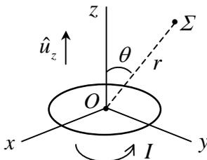
Fig. 10.12. A magnetic dipole a distance  $r$  from the observation point  $\Sigma$ .
