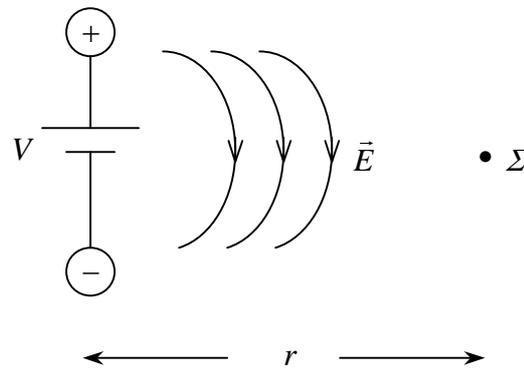
Fig. 10.11. An example of an oscillating electric dipole; the observation point  $\Sigma$  is a distance  $r$  from the dipole.
