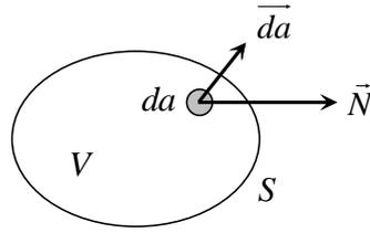
Fig. 9.4. Poynting vector on a closed surface  $S$  enclosing a volume  $V$ .
