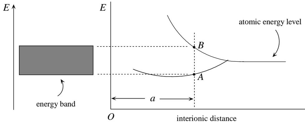
Fig. 1.6. Formation of an energy band in a crystal.
