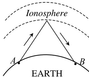
Fig. 10.13. Transmission of a radio wave by reflection on the Ionosphere.
