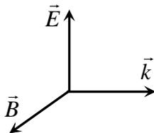
Fig. 10.5. Relative directions of the electromagnetic field and the wave vector. The latter vector determines the direction of propagation of the wave.
