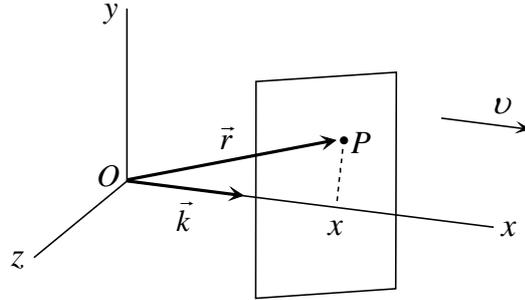
Fig. 10.3. Wave surface of a plane wave traveling in the  $+x$ -direction.
