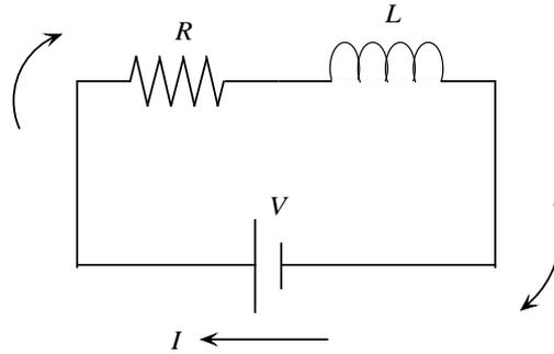
Fig. 9.9. A circuit having total resistance  $R$  and inductance  $L$ .
