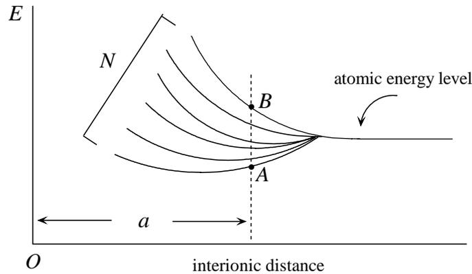
Fig. 1.5. Splitting of an atomic energy level into  $N$  crystalline levels.
