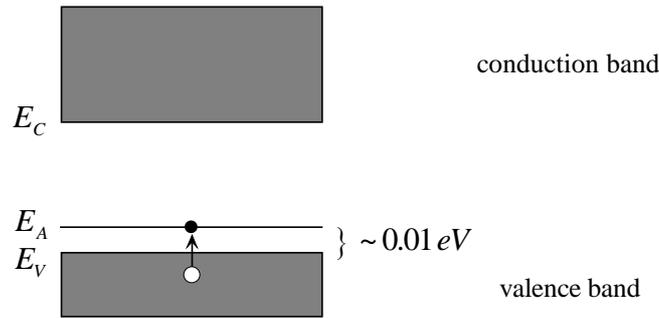
Fig. 2.10. Band structure of a  $p$ -type semiconductor.
