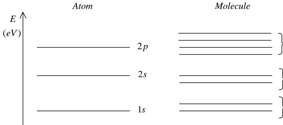
Fig. 1.4. Energy-level diagrams for an atom (left) and the corresponding diatomic molecule (right).
