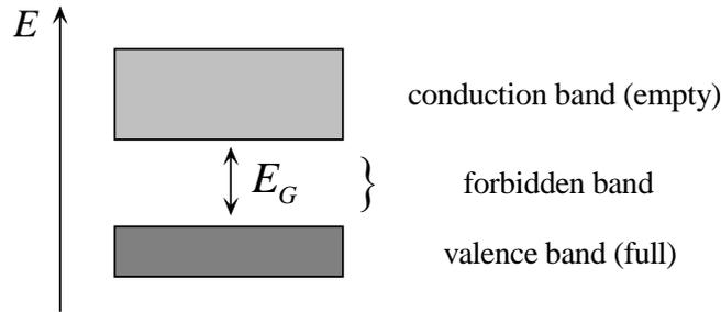
Fig. 1.9. Valence, conduction, and forbidden bands; the energy gap is  $E_G$ .
