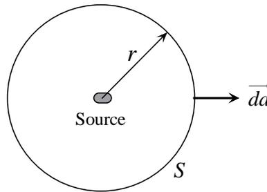
Fig. 10.7. A source of e/m radiation at the center of a spherical surface  $S$  of radius  $r$ .
