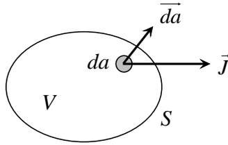
Fig. 6.3. Current density on a closed surface  $S$  enclosing a volume  $V$ .
