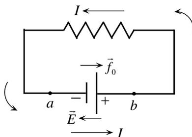
Fig. 9.6. An ideal battery connected to an external resistor. The circuit is positively oriented in the direction of the current.
