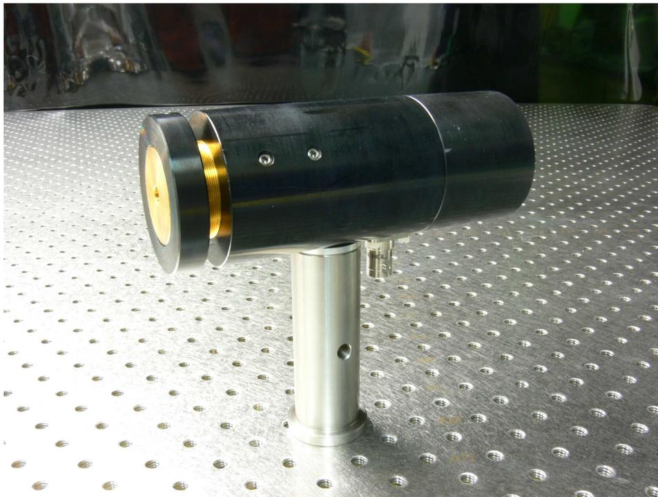
Here is the same cavity disassembled. On the left you can see one of the mirrors mounted on a threaded barrel. The barrel is used to adjust the cavity length to match precisely the mirror curvatures. The other mirror is attached to the right-hand side of the main body on a tubular piezo stack, which gives a total displacement of  $\sim 1$   $\mu\text{m}$  for a 0–15 V control signal. The mirror cover on the right contains a photodiode to monitor the transmitted light.
