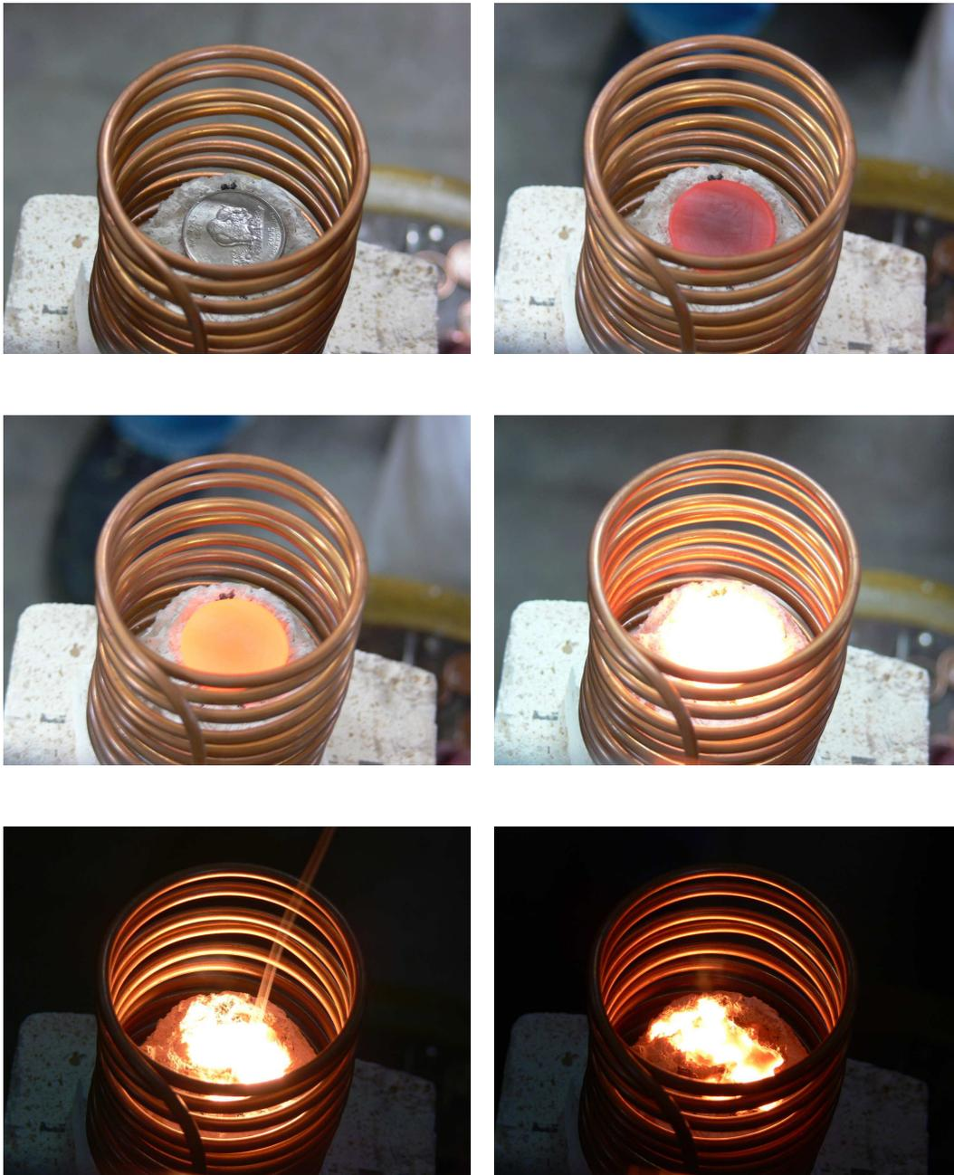
Here is a movie of the heating process, where you can see the heat flowing in from the outside of the quarter to the inside.
