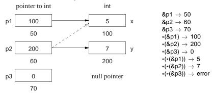
A pointer/reference may point to the same memory address as another pointer/reference (dashed line). Also, dereferencing the null pointer is an error because no variable is allocated at address 0.
