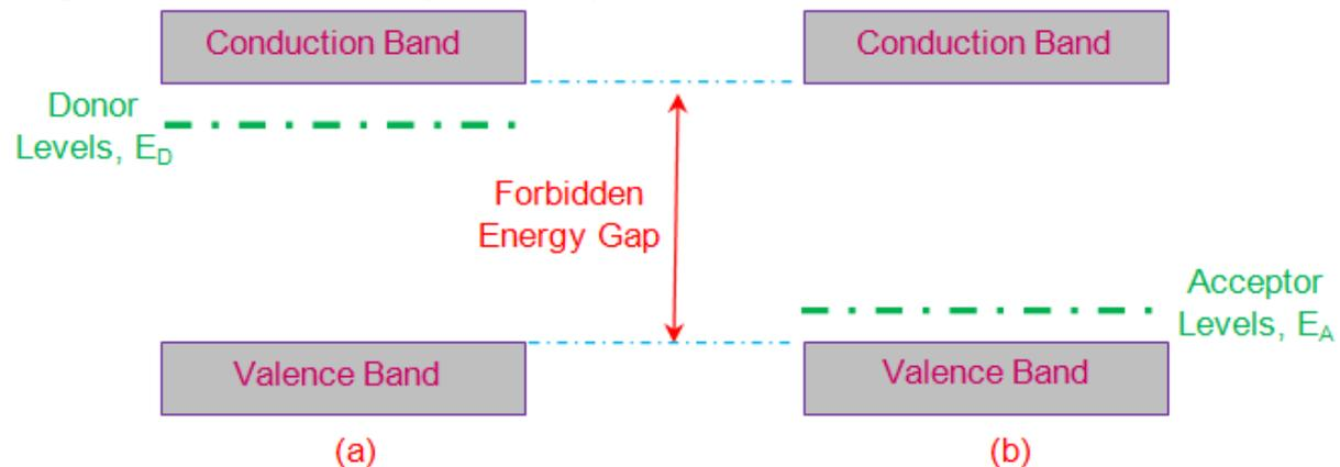
Figure 2 Energy Band Diagram of (a) *n*-type Extrinsic Semiconductor
