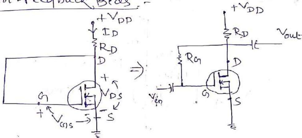
Two figures show this biasing technique. As for n-channel EMOsFET, A high resistance  $R_G$  is connected between the drain & gate ( $\because I_G = 0$ ), therefore, voltage drop across  $R_G = 0V$  and the gate will be at same potential as the drain.
