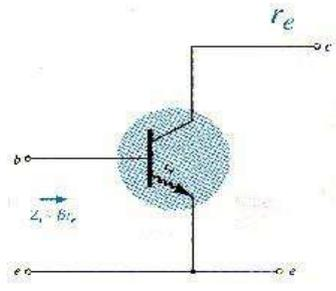
Fig5-10  $r_e$  on input impedance
