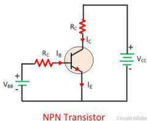
The value of collector emitter voltage at any given time will be
