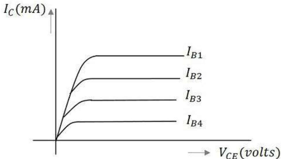
In the above figure, the output characteristics are drawn between collector current  $I_C$  and collector voltage  $V_{CE}$  for different values of base current  $I_B$ . These are considered here for different input values to obtain different output curves.
