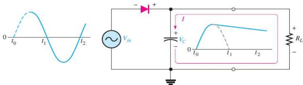
(b) The capacitor discharges through  $R_L$  after peak of positive alternation when the diode is reverse-biased. This discharging occurs during the portion of the input voltage indicated by the solid dark blue curve.
