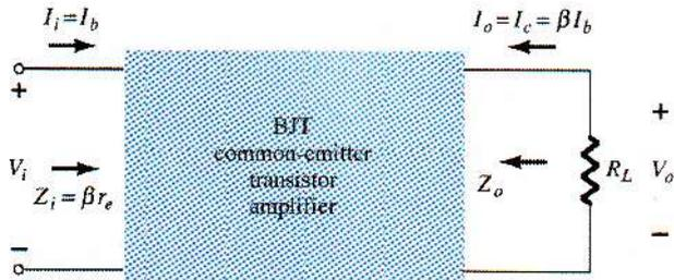
Fig 5-12 Determining  $A_v$  &  $A_i$  for the CE
