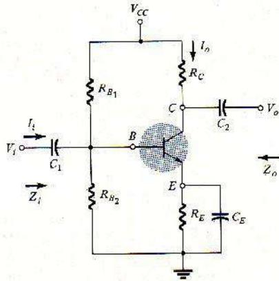
Fig6-7 voltage divider bias Configuration
