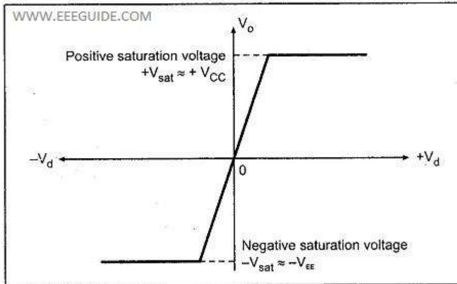
Fig. 2.7 Ideal voltage transfer curve
