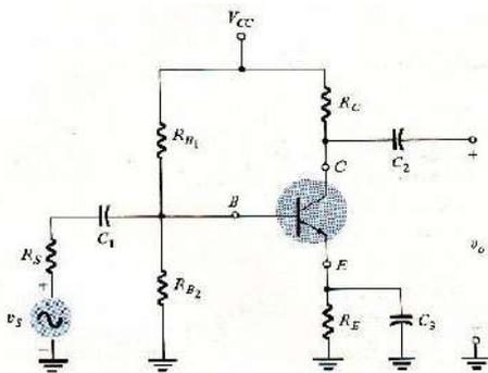
Fig 5-1 Transistor circuit under examination
