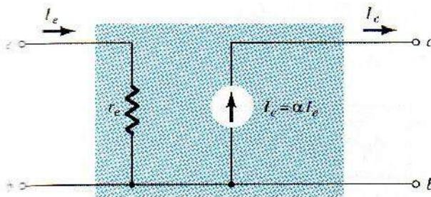
Fig 5-5 CB  $r_e$  equivalent circuit
