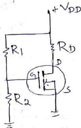
$$I_G = 0, \text{ so } V_{GS} = \frac{V_{DD}}{R_1 + R_2} \times R_2$$
