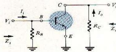
Fig 6-2 removal of effects of  $V_{CC}$ ,  $C_1$ ,  $C_2$
