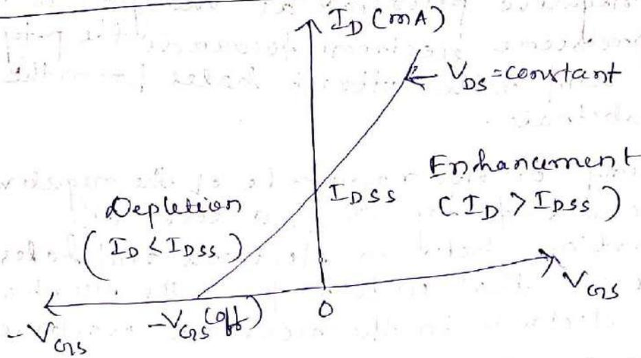
$(I_D, V_G, V_{GS}) \Rightarrow$  Transfer characteristics
