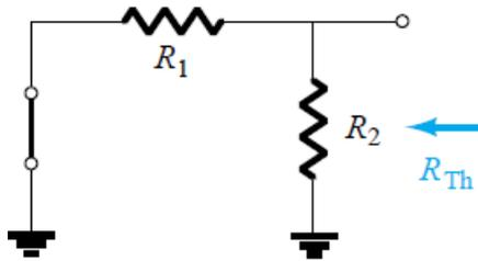
$$R_{Th} = R_1 \parallel R_2$$
