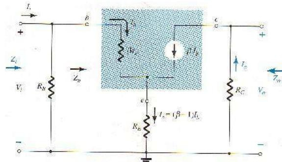
Fig6-11  $r_e$  equivalent for circuit of fig6-10
