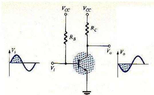
Fig-5 180° phase shift between input & output
