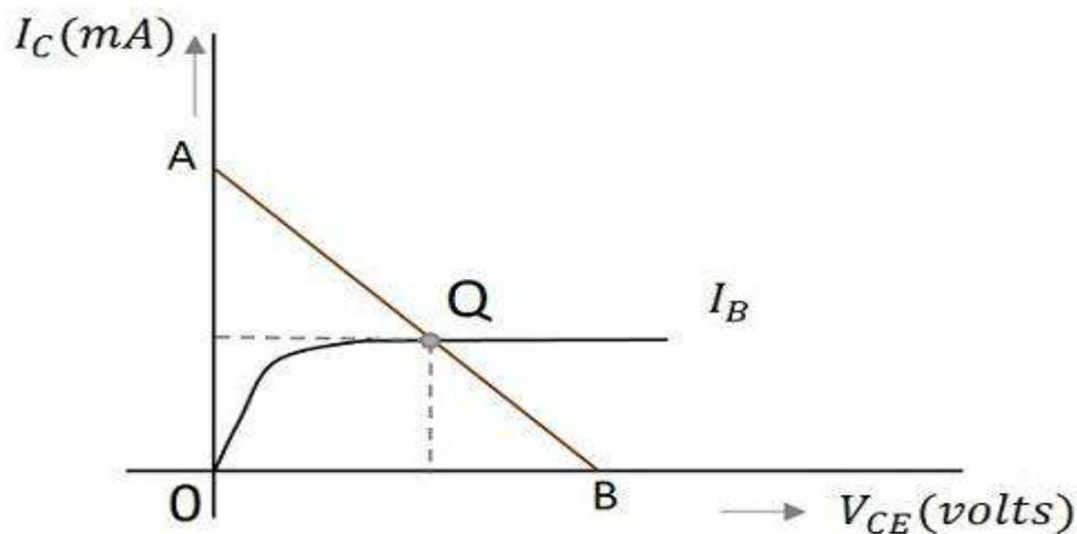
The load line has to be drawn in order to obtain the Q-point. A transistor acts as a good amplifier when it is in active region and when it is made to operate at Q-point, faithful amplification is achieved.
