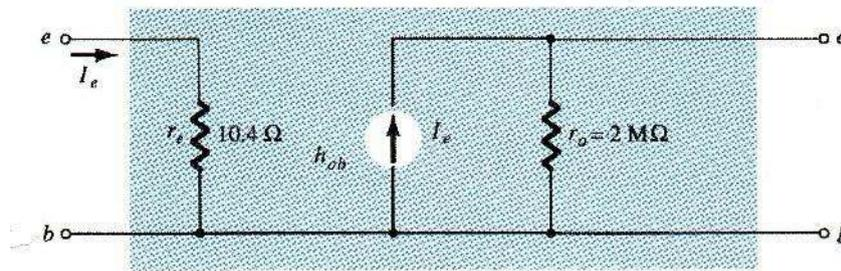
Fig5-24 CB  $r_e$  model of Ex 5:
