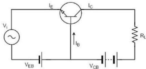
The low resistance in input circuit, lets any small change in input signal to result in an appreciable change in the output. The emitter current caused by the input signal contributes the collector current, which when flows through the load resistor  $R_L$ , results in a large voltage drop across it. Thus a small input voltage results in a large output voltage, which shows that the transistor works as an amplifier.
