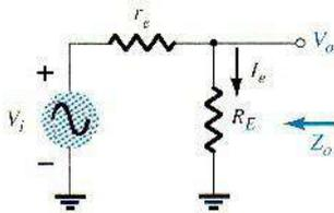
Fig6-18 the output impedance for Emitter-follower
