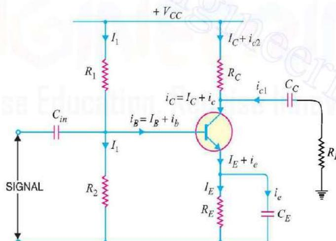
(iii) **Emitter bypass capacitor  $C_E$ .** An emitter bypass capacitor  $C_E (\approx 100\mu F)$  is used in parallel with  $R_E$  to provide a low reactance path to the amplified a.c. signal. If it is not used, then amplified a.c. signal flowing through  $R_E$  will cause a voltage drop across it, thereby reducing the output voltage.
