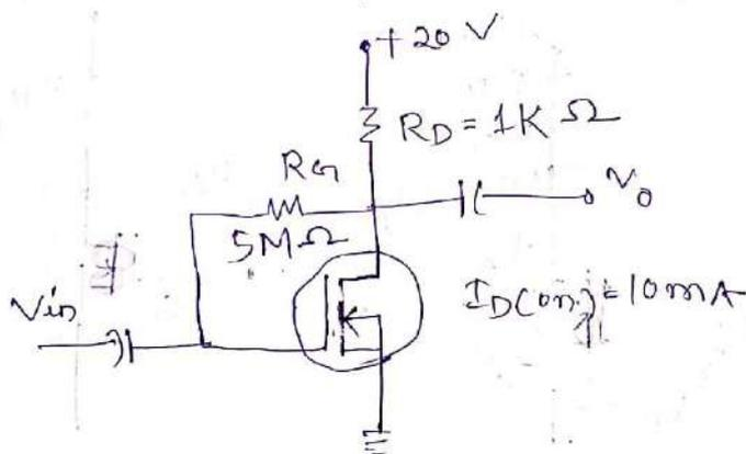
Ans -  $V_{GS} = V_{DS}$  (as source is grounded and  $R_G$  is in  $M\Omega$  so  $I_G = 0$ )
