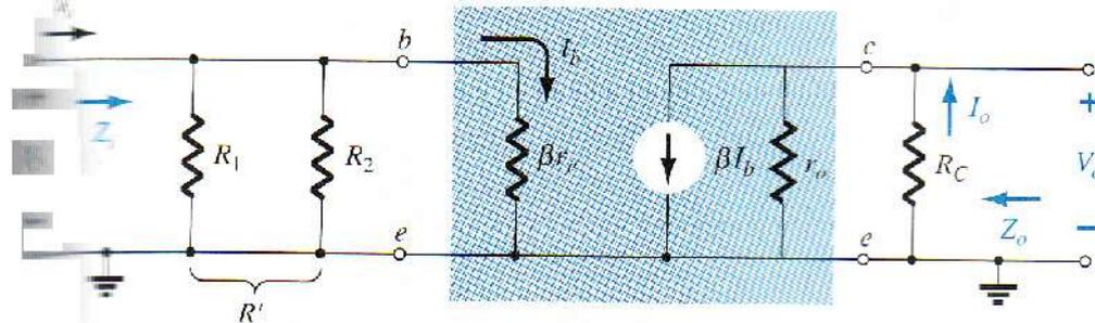
Fig6-8 substituting the  $r_e$  equivalent circuit into the ac equivalent network
