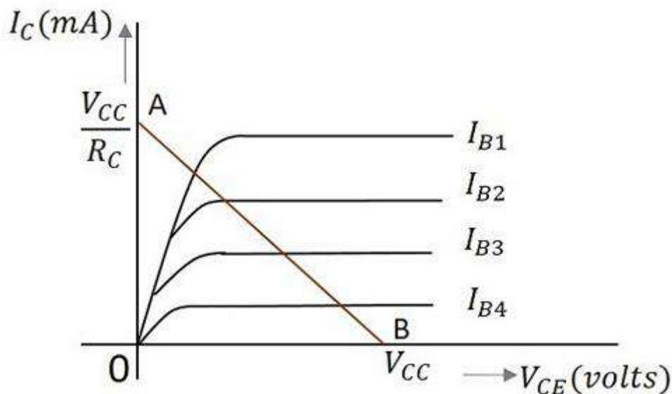
To obtain the load line, the two end points of the straight line are to be determined. Let those two points be A and B.
