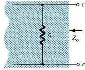
Fig 5-11  $r_o$  equivalent circuit
