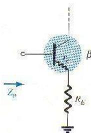
Fig6-12 the input impedance of an un bypassed CE
