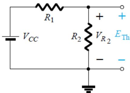
$E_{Th}$ : The voltage source  $V_{CC}$  is returned to the network and the open-circuit Thévenin voltage
