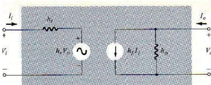
Fig5-17 complete hybrid equivalent circuit
