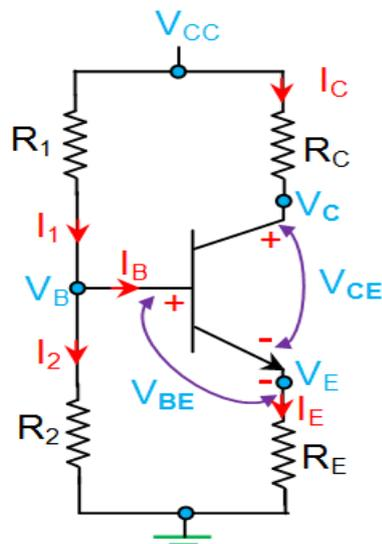
Figure 7 Voltage Divider Bias Circuit
