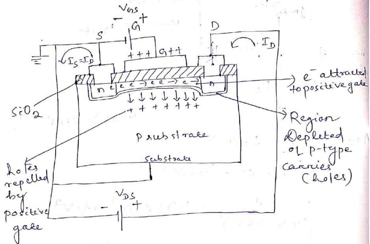
→ The level of  $V_{GS}$  that results in significant increase in drain current is called as 'THRESHOLD VOLTAGE' and symbol is  $V_T$ .
