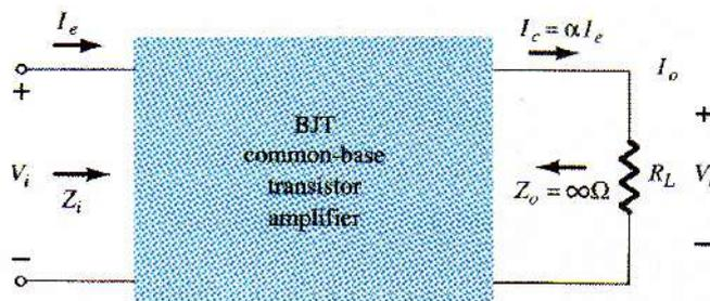
Fig 5-6  $A_v = V_o/V_i$  for CB
