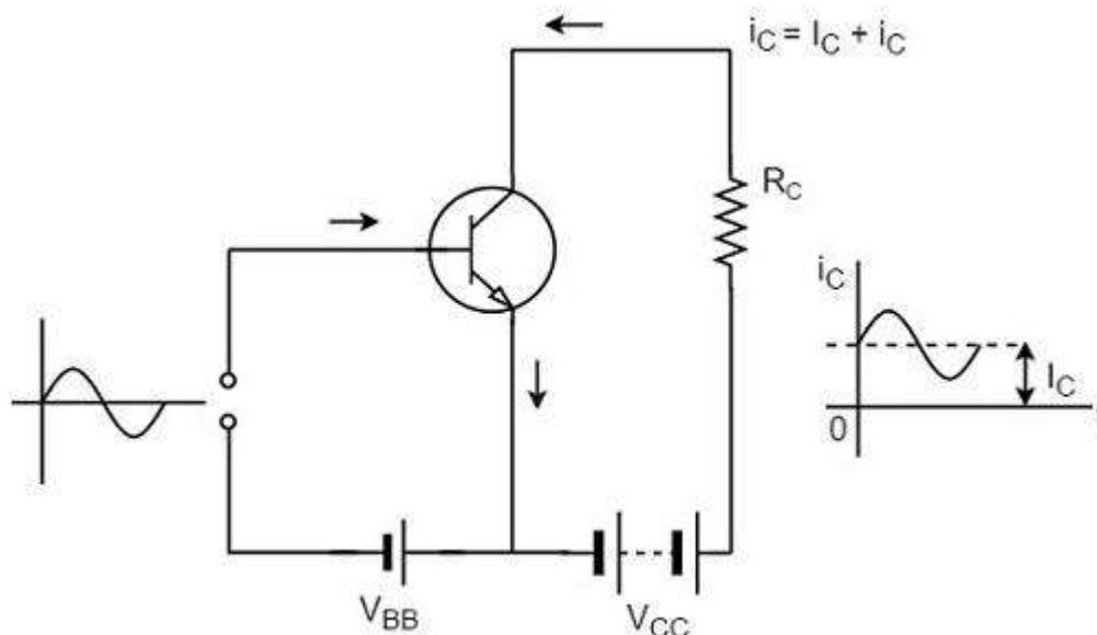
Hence for faithful amplification, proper zero signal collector current must flow. The value of zero signal collector current should be at least equal to the maximum collector current due to the signal alone.
