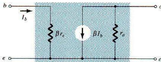
Fig 5-13  $r_e$  model for the CE configuration
