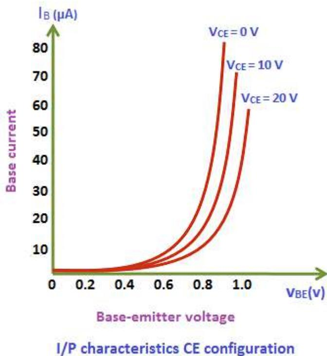
$I_B$  (Base Current) is the input current,  $V_{BE}$  (Base – Emitter Voltage) is the input voltage for CE (Common Emitter) mode. So, the input characteristics for CE mode will be the relation between  $I_B$  and  $V_{BE}$  with  $V_{CE}$  as parameter. The typical
