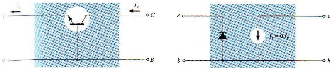
Fig 5-7 approximate model for a CB npn transistor configuration
