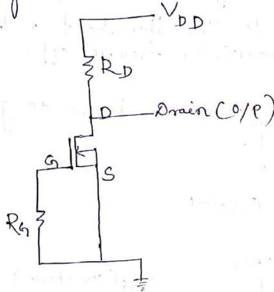
Here  $V_{GS} = 0$  as no voltage difference from gate to source or zero biasing is given.
