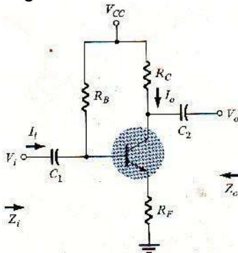
Fig6-10 CE Un bypassed configuration
