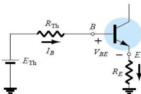
$$E_{Th} - I_B R_{Th} - V_{BE} - I_E R_E = 0$$
