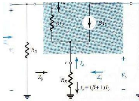
Fig6-17 re model for network of fig 6-16
