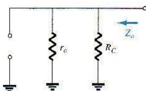
Fig 6-4 Determining  $Z_o$  for the network
