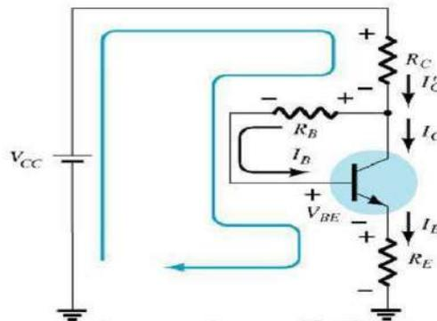
**Applying KVL for Input Loop:**
