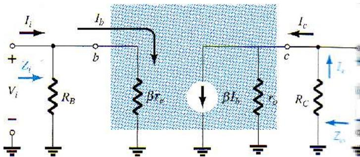
Fig 6-3  $r_e$  model to the network
