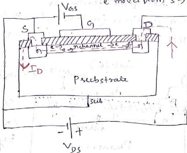
→ When gate-to-source voltage is set to ( $V_{GS}=0$ ) zero and a positive voltage  $V_{DS} > 0$  is applied, then as drain is at more potential as compared to source, so, the result is an attraction for the positive potential at the drain by free electrons of the n channel.
