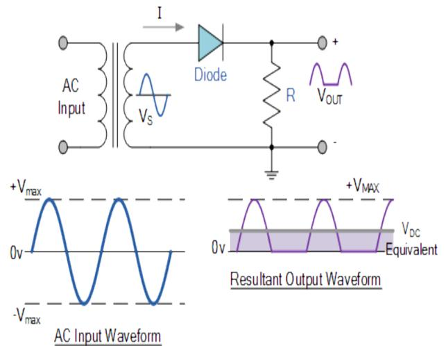
During the negative half cycle, the anode will become negative and the cathode will become positive, which is known as reverse bias. So the diode will block the negative cycle.
