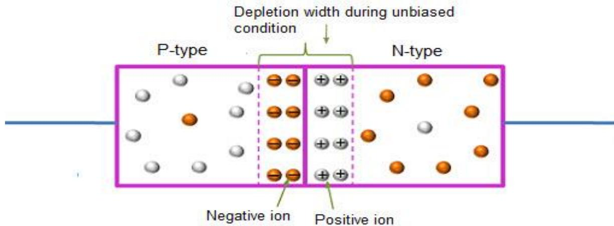
This pn junction does not allow flow of current. To make it suitable for electronics circuits we need to biasing (applying external voltage) pn-diode. There are two ways of biasing pn-diode (i) Forward biasing
