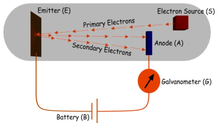
velocity striking electrons, transferred to the free electrons on the metal surface. Thus the free electrons may get sufficient kinetic energy to overcome the surface barrier and knocked out from the surface & start electron emission.
