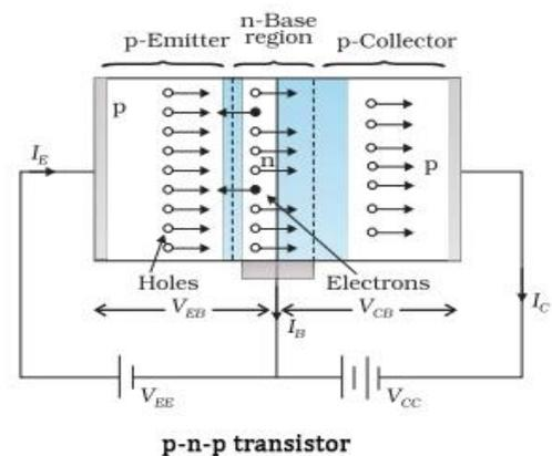
The ratio of change in collector current ( $\Delta I_C$ ) to the change in emitter current ( $\Delta I_E$ ) at constant collector-base voltage ( $V_{CB}$ ) is known as **current amplification factor** in common base (CB) arrangement. i.e.  $\alpha = \Delta I_C / \Delta I_E$
