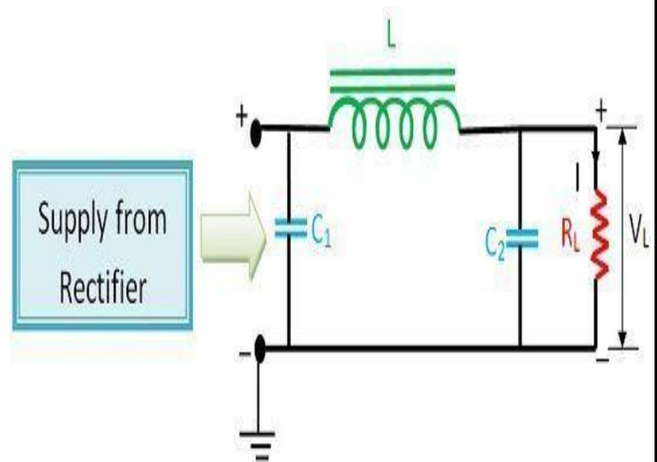
in series and another filter capacitor  $C_2$  connected across the load. The shape of the circuit diagram of this filter circuit appears like Greek letter  $\pi$  ( $\pi$ ) and hence the name  $\pi$ -filter.
