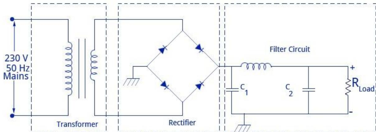
A small step down transformer is used to reduce the voltage level as the device needed. The output of the transformer is a pulsating AC voltage which is fed into a rectifier circuit. The rectifier converts it and its output is pulsating DC. Again this output is fed to a filter circuit as input. This filter circuit then removes the AC components present if any and gives a DC voltage as required by the electronic circuit.
