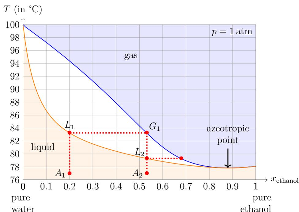
Figure 8.3: Principle of distillation.
