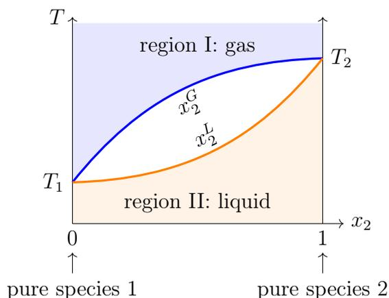
Figure 8.1: An isobar phase diagram of a typical binary solution. For the pressure considered,  $T_1$  is the liquid/gas coexistence temperature of species 1 alone and  $T_2$  is the liquid/gas coexistence temperature of species 2 alone.
