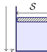
For a transformation where the external pressure is constant, we have of course  $W = -p_{\text{ext}} \Delta V = -\Delta(p_{\text{ext}} V)$ . When the external pressure is constant and the system is in mechanical equilibrium at the initial ( $p_{\text{ext}} = p_{\text{initial}}$ ) and final ( $p_{\text{ext}} = p_{\text{final}}$ ) stages, the work of the pressure forces is then  $W = -\Delta(pV)$  and, if there are no other forces producing work,
