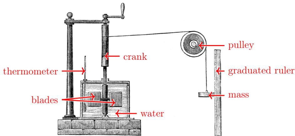
Figure 2.1: The Joule apparatus to establish heat/energy equivalence.
