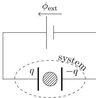
A system made of a sample placed between the armatures of a capacitor is considered. A voltage  $\phi_{\text{ext}}$  is applied to this capacitor by a generator; it is this generator (placed outside the system) that delivers the work. During a transformation that, for example, changes the capacity of the capacitor, the electric charge on its plates changes. The work received is then
