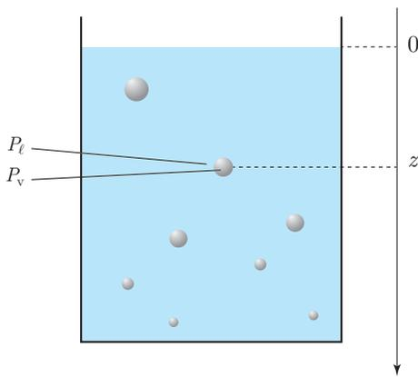
Schematic of boiling in a liquid.
