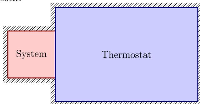
A thermostat is an ideal system, considered so big that its temperature does not change, even when it receives (or gives) energy in the form of heat (see frame 3.4). In particular, the thermostat imposes its temperature on the system. We consider that the system can only exchange heat with the thermostat, and the {system + thermostat} entity is isolated.
