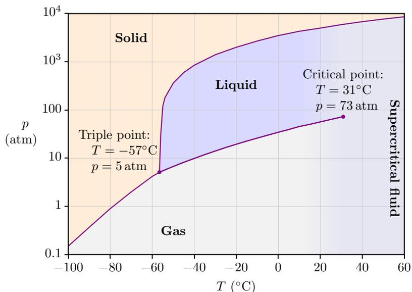
Figure 7.1: Phase diagram of CO<sub>2</sub>. Note the logarithmic scale of the pressure which makes it possible to display on the same figure a very wide range of pressures.
