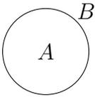
The fluid  $A$  is enclosed in an elastic membrane (balloon, soap bubble, *etc.*) which is immersed in the fluid  $B$  (typically the atmosphere). Then  $p_A > p_B$ , and the difference between the two pressures depends on the elastic properties of the membrane and its radius of curvature.
