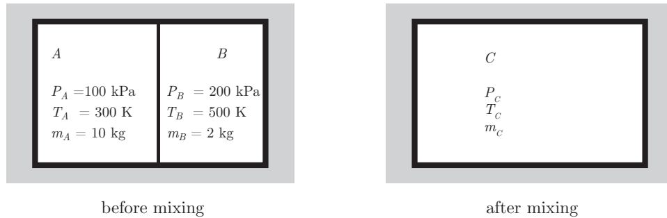
Figure 6.30: Schematic for a globally adiabatic thermo-mechanical mixing problem.
